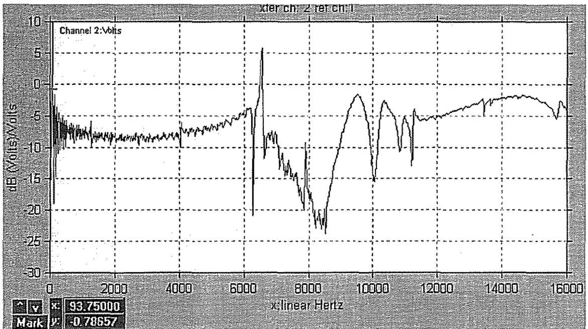
Figure 8: Frequency response of force transducer in the fixed condition (vertical impact).
