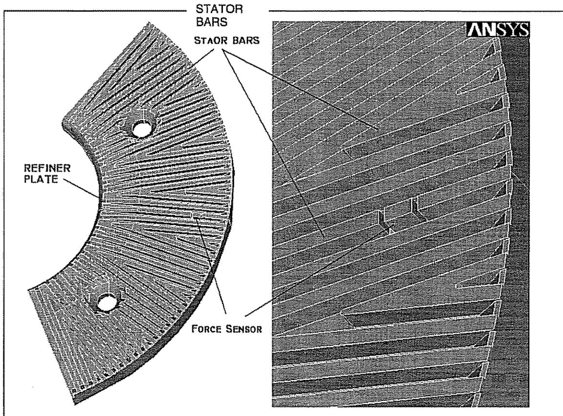
Figure 2: Schematic of force transducer installed in refiner plate segment.
