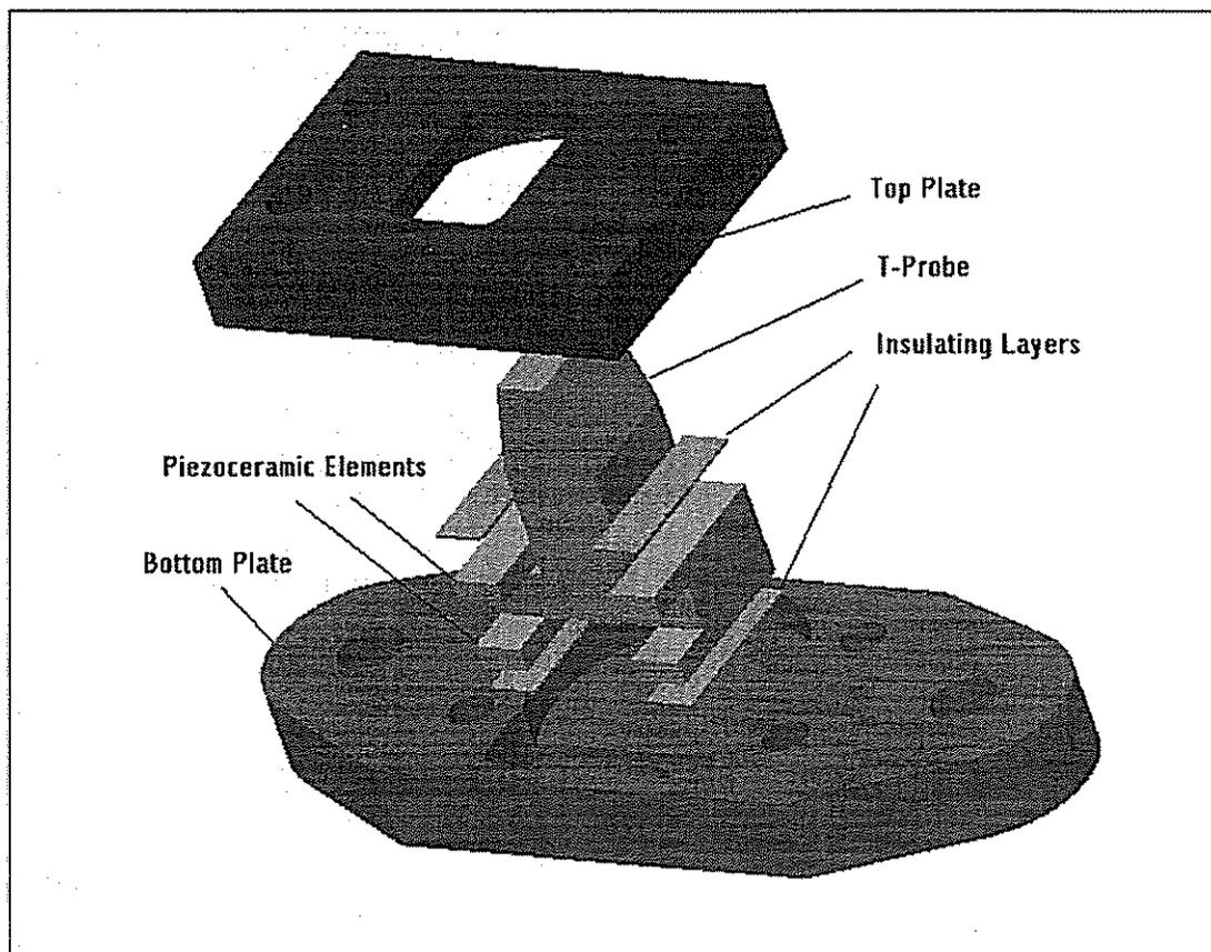
Figure 4: Exploded isometric view of the transducer.
