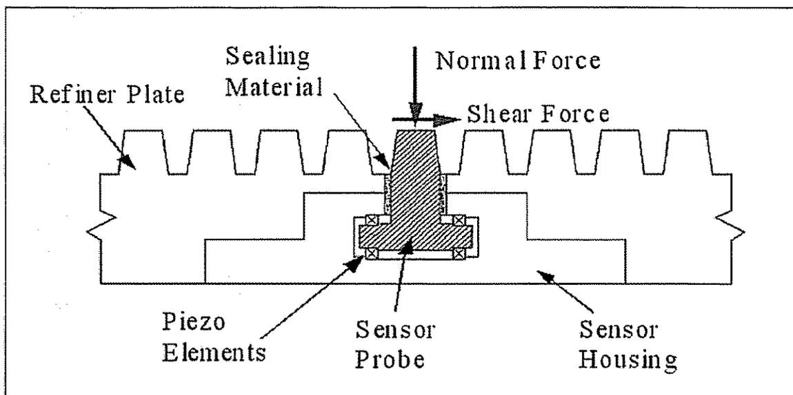
Figure 3: Schematic cross-section of force transducer.
