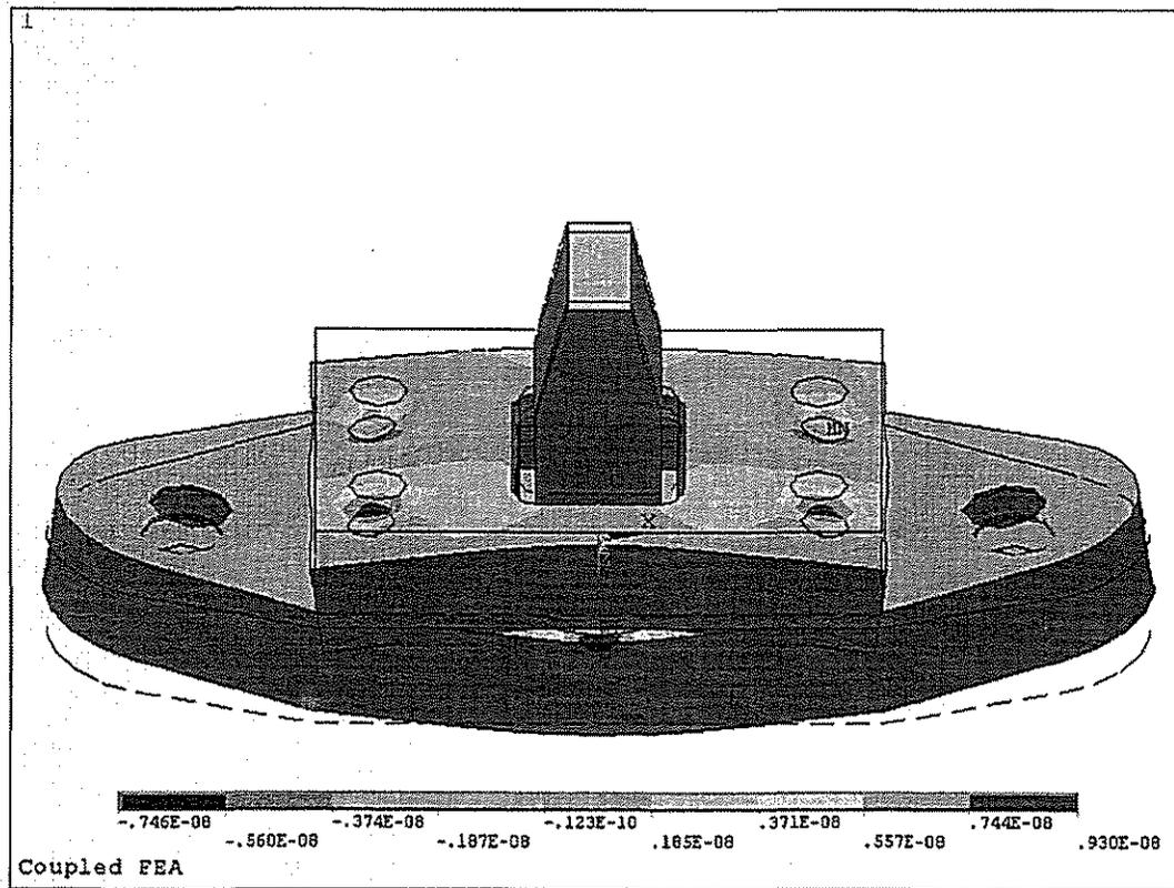
Figure 6: Transducer deformation due to preload ( $\Delta T = -1.47 \text{ } ^\circ\text{C}$ )
