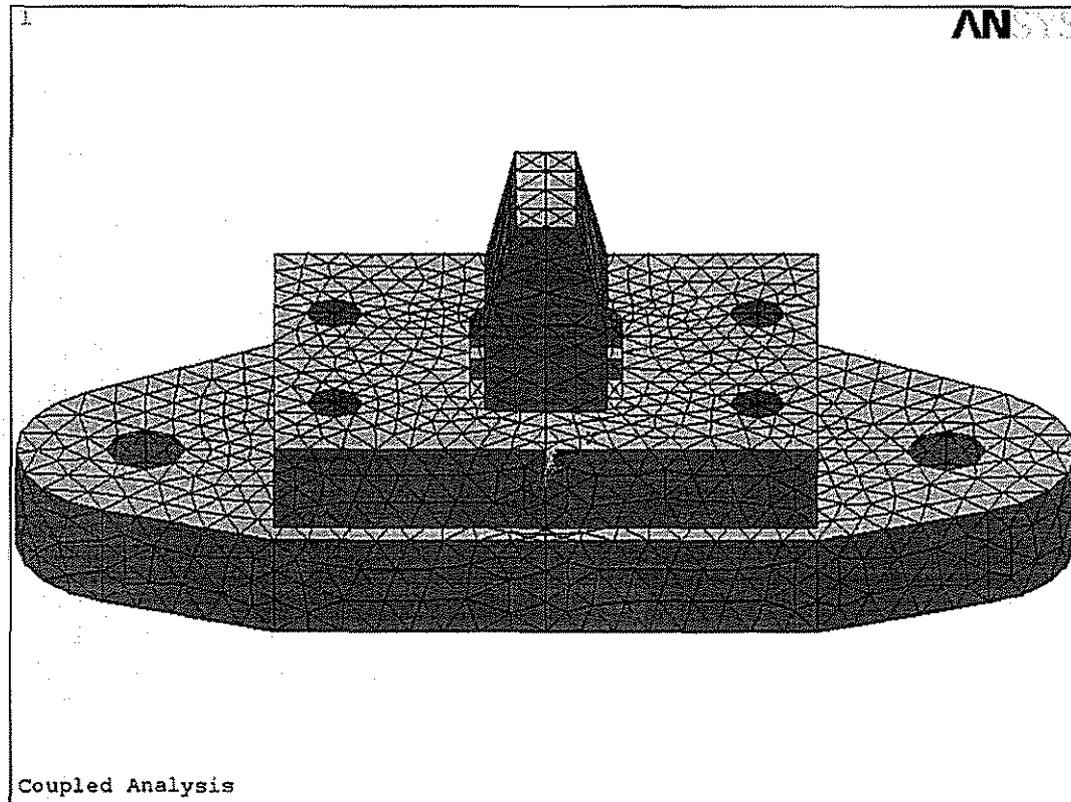
Figure 5: Finite element model of force transducer.
