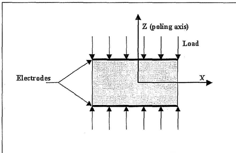
Figure 1: Load Diagram of a piezoelectric element.
