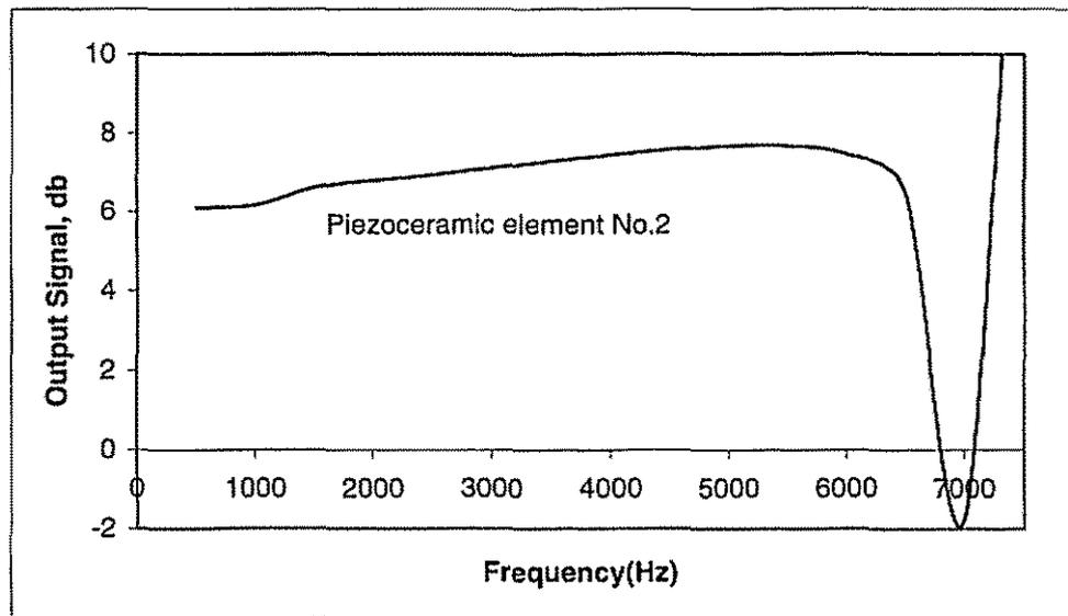
Figure 9: Piezoelectric elements outputs based on Finite Element harmonic analysis.
