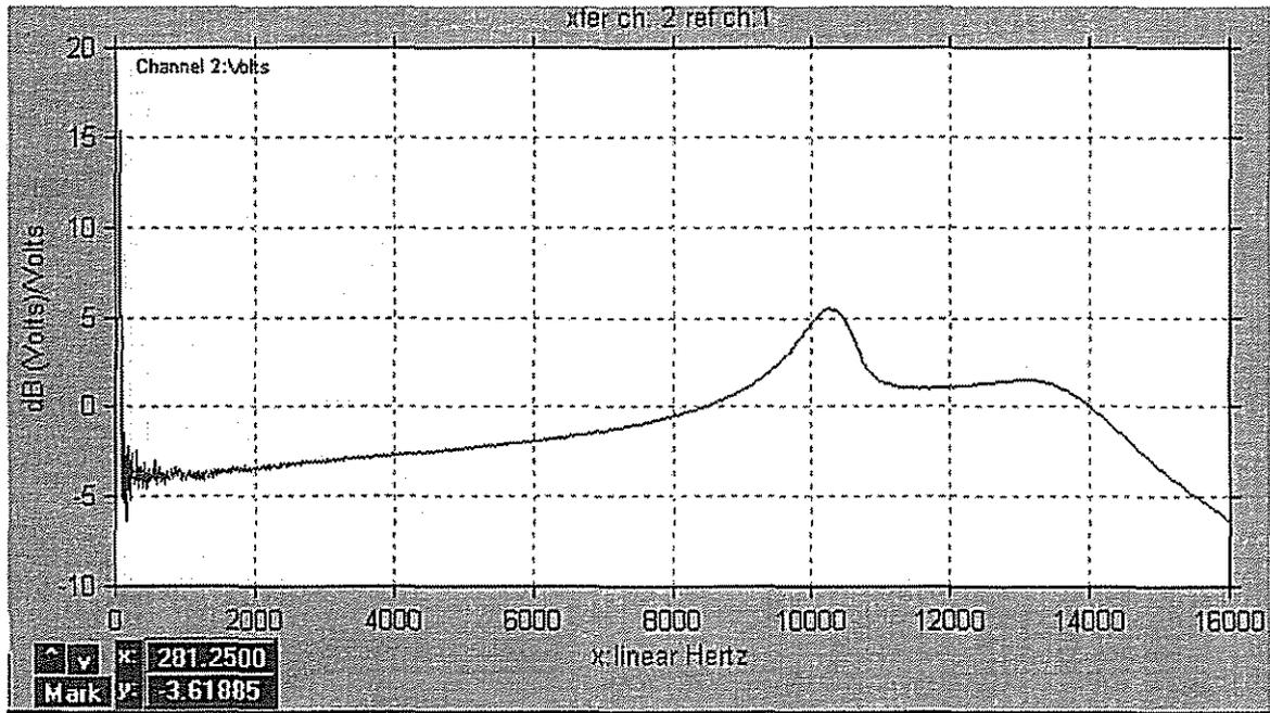
Figure 7: Frequency response of force transducer in the free condition (vertical impact).
