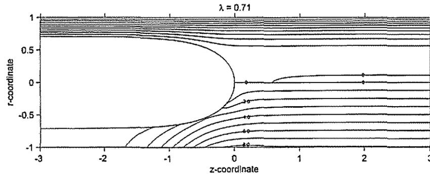
Fig. 3 Distribution of streamline and vorticity for  $\lambda = 0.71$
