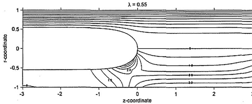
Fig. 2 Distribution of streamline and vorticity for  $\lambda = 0.55$
