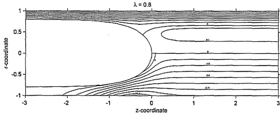
Fig. 4 Distribution of streamline and vorticity for  $\lambda = 0.8$
