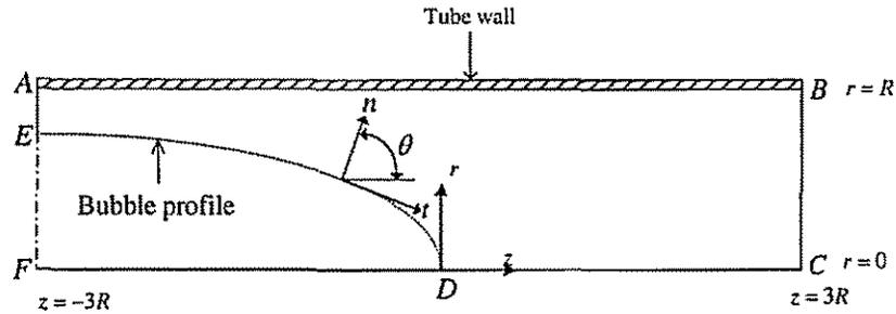
Fig. 1 Physical diagram showing the coordinate system used in the study of a gas bubble steadily expelling viscous fluid.
