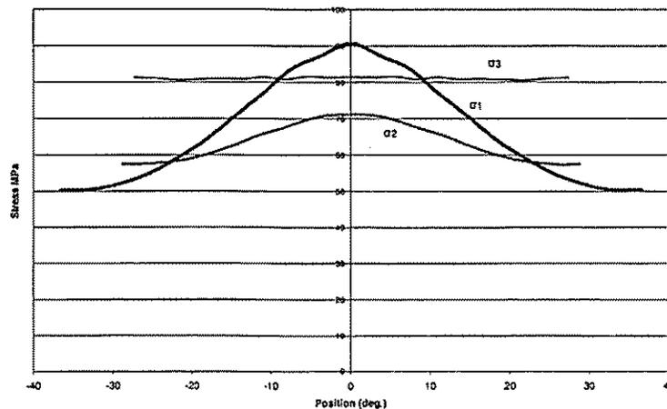
Fig. 7 : Worm Tensile Fillet Stress vs. Angular Position for all contact lines
