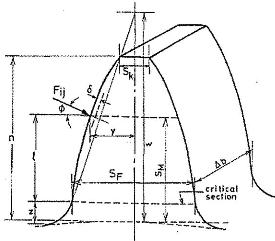
Fig. 2 : Tooth deflection and fillet stress parameters
