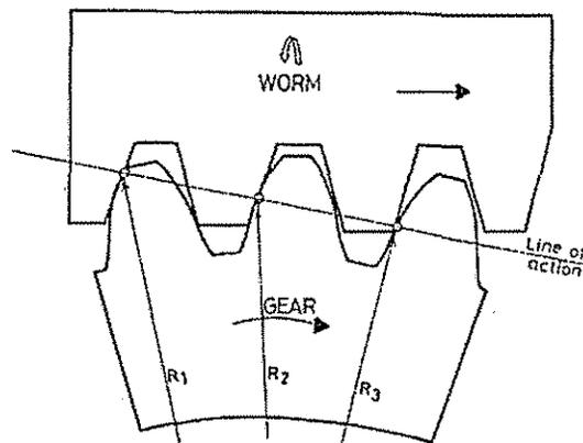
Fig. 3 : Line of action intersecting teeth of a slice
