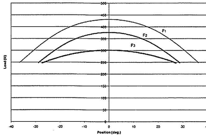
Fig. 6 : Load distribution on contact lines
