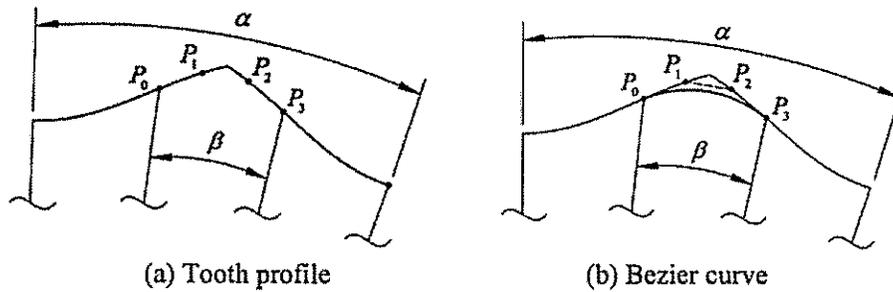
Fig. 11 Single tooth profile for epicycloidal profiles (example 1, case 2)
