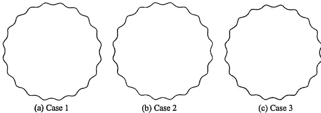
Fig. 19 Epicycloidal profiles after addendum modified for example 2
