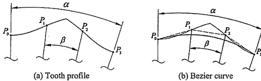
Fig. 10 Single tooth profile for epicycloidal profiles (example 1, case 1)
