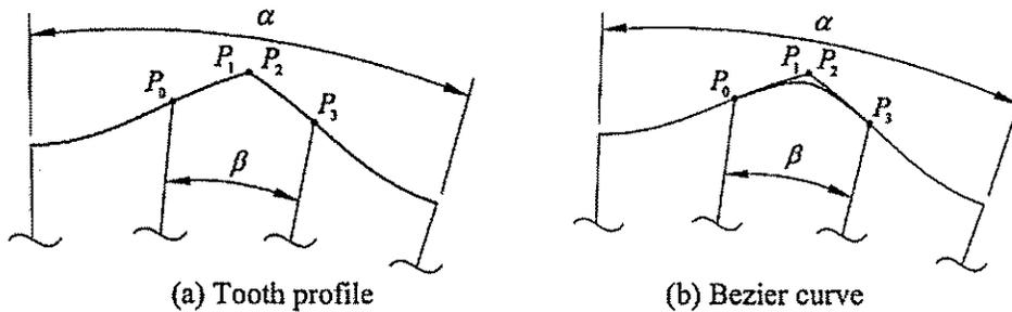
Fig. 12 Single tooth profile for epicycloidal profiles (example 1, case 3)
