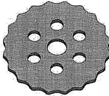
Fig. 21 Solid modeling after addendum modified for example 2 (case3)
