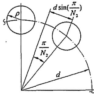
Fig. 4 Geometrical relationships of cylindrical meshing elements
