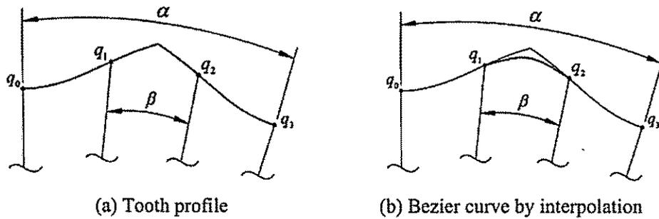
Fig. 15 Single tooth profile for epicycloidal profiles (example 2, case 1)
