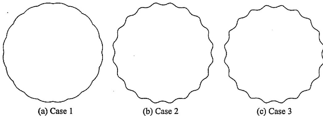
Fig. 14 Epicycloidal profiles after addendum modified for example 1
