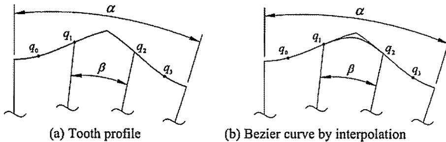
Fig. 16 Single tooth profile for epicycloidal profiles (example 2, case 2)
