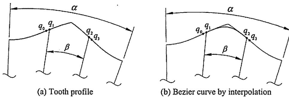
Fig. 17 Single tooth profile for epicycloidal profile (example 2, case 3)
