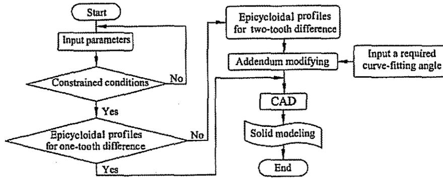
Fig. 5 Flow chart of the design and addendum modifying for cycloid drives
