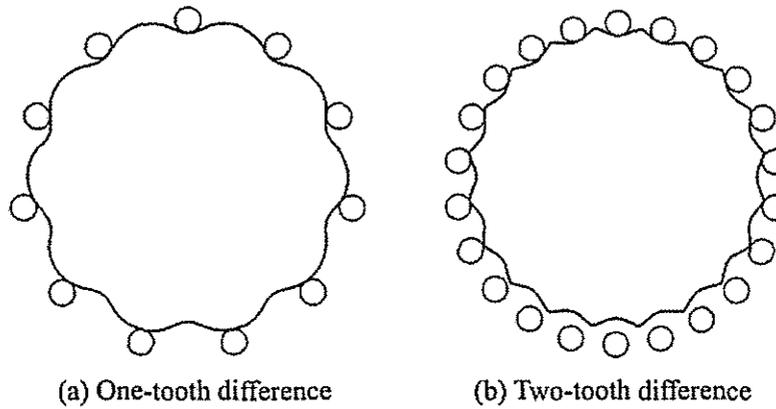
Fig. 6 Epicycloidal profiles and cylindrical meshing elements
