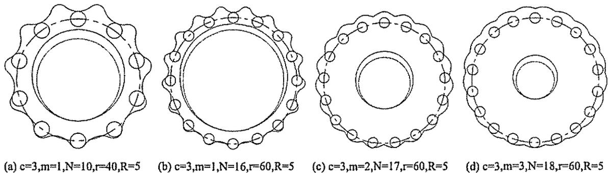
Fig. 6 Design results of pin wheel hypotrochoid meshing
