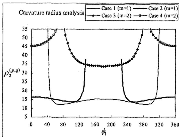
Fig. 10 Radius of curvature of trochoidal curve
