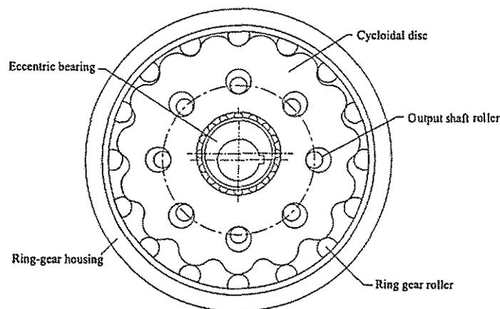
Fig. 1 Schematic of a cycloidal speed reducer
