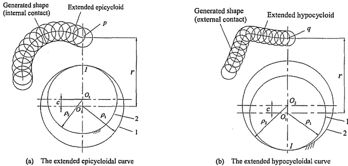
Fig. 3 Generation of trochoidal curve
