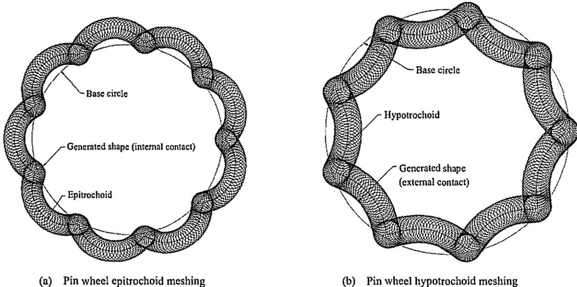
Fig. 2 Basic idea of cycloidal speed reducer
