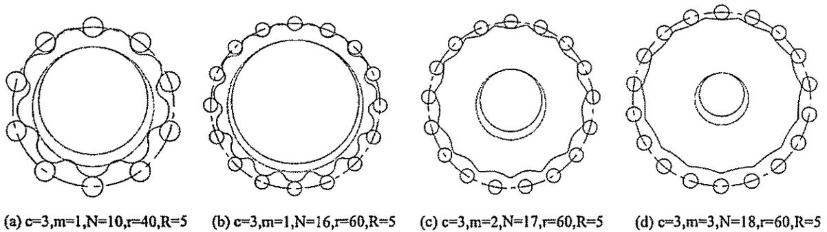
Fig. 5 Design results of pin wheel epitrochoid meshing
