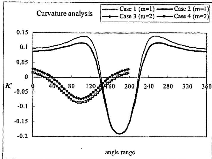
Fig. 11 Curvature of cycloidal wheel
