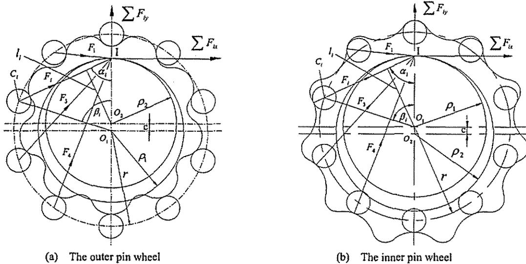
Fig. 7 Contact forces of the cycloidal speed reducer
