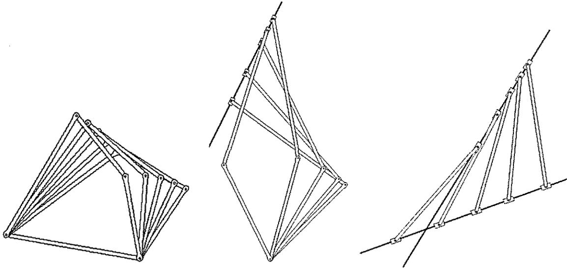
Figure 2: All possible four-bar mechanisms: a general one, a slider crank and a double slider mechanism
