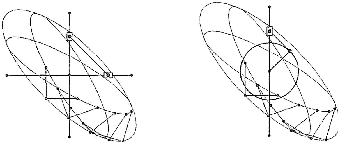
Figure 7: A double slider and a slider crank mechanism that guide  $\Sigma$  through the given poses
