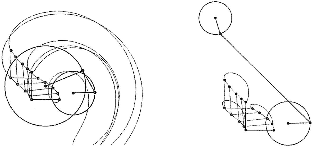
Figure 4: Two out of the six real general four-bar mechanisms that guide  $\Sigma$  through the given poses
