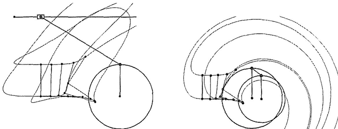
Figure 5: A slider crank and a general four-bar mechanism that guide  $\Sigma$  through the given poses
