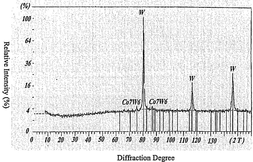
Fig 5: Relative intensity versus diffraction degree for sintered Tungsten specimen (W-1%Co).
