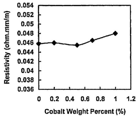
Fig 7: Resistivity of W-Cu-Co specimens versus cobalt weight percent
