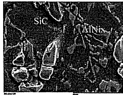
Figure 5: Microstructure du composite GrA-Ni® 10S-4G (X 1200).
