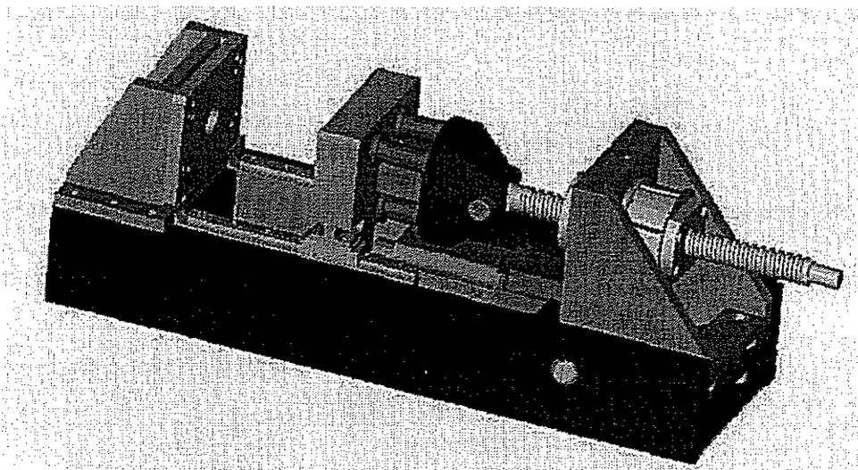
Fig. 6 Assembly model of tiebarless clamping unit
