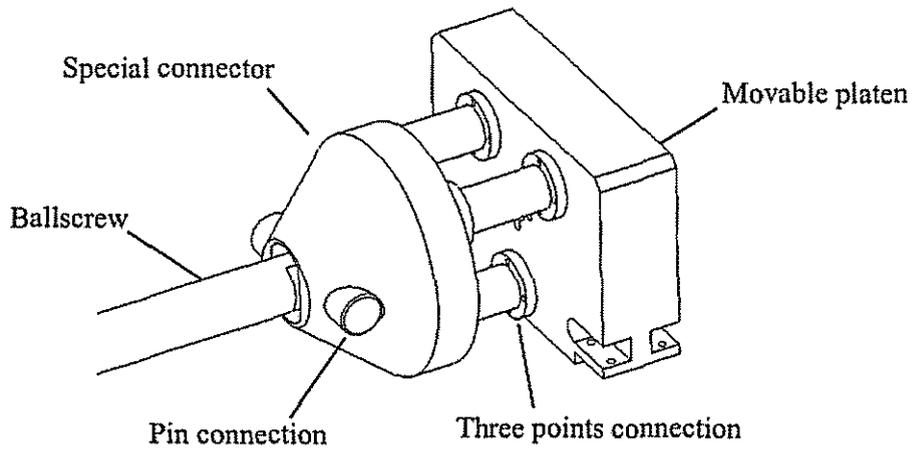
Fig. 3 Connector between ballscrew and movable platen
