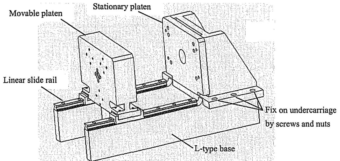
Fig. 2 Stationary platen, movable platen and linear slide rail
