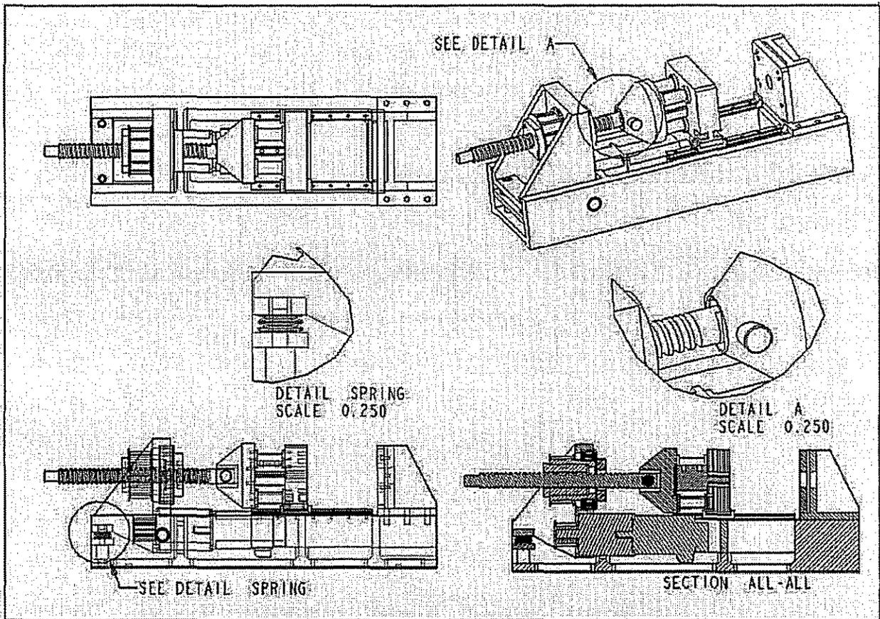
Fig. 1 Detail design drawing of tiebarless clamping unit
