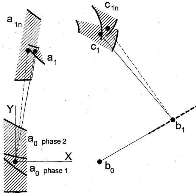
**Figure 5.** Tolerance regions and pivot selections for 5-bar motion generator
