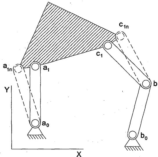
**Figure 2.** Five-bar motion generator with adjustable moving pivots
