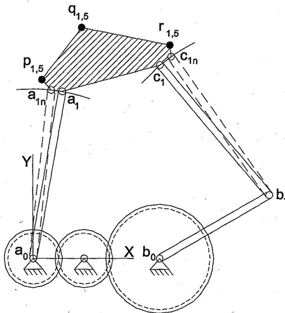
**Figure 6.** Synthesized adjustable 5-bar mechanism
