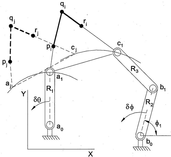
**Figure 4.** Planar five-bar mechanism with driving link angles  $\theta$  and  $\phi$  and rigid-body points  $p$ ,  $q$  and  $r$
