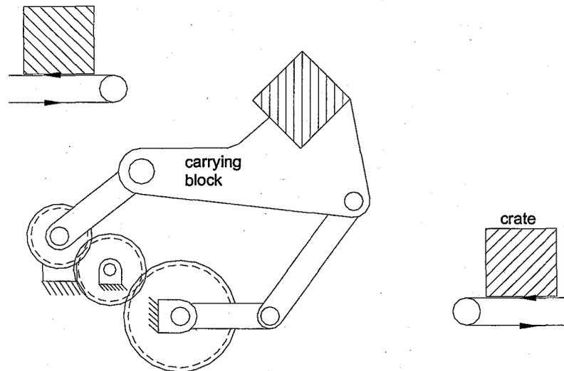
Figure 1. Five-bar mechanism used in package handling
