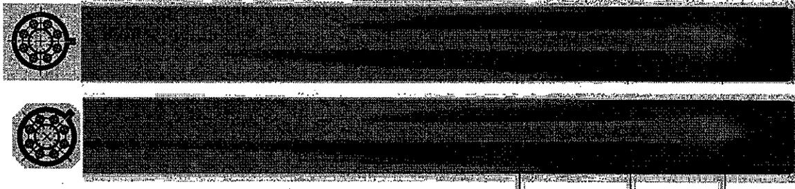
Figure 3: Pressure contours along missile body at AoA = 17 deg. for flow effectors placed at 270 deg. (top) and 225 deg. (bottom) angular positions. Nose cone is on righthand side of the diagram.
