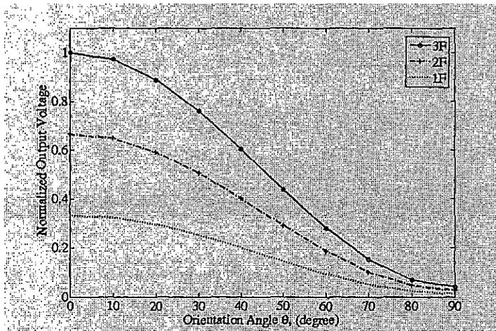
**Figure 3.** The normalized output voltage of the uniaxial piezoelectric PVDF film for different applied loads
