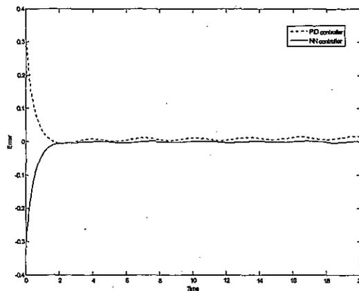
Fig. 9 Comparison of tracking errors between the two control schemes
