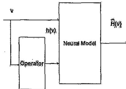
Fig. 1. Expanded input space for modeling hysteresis
