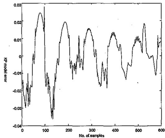
Fig. 5 The validation error of the KP model
