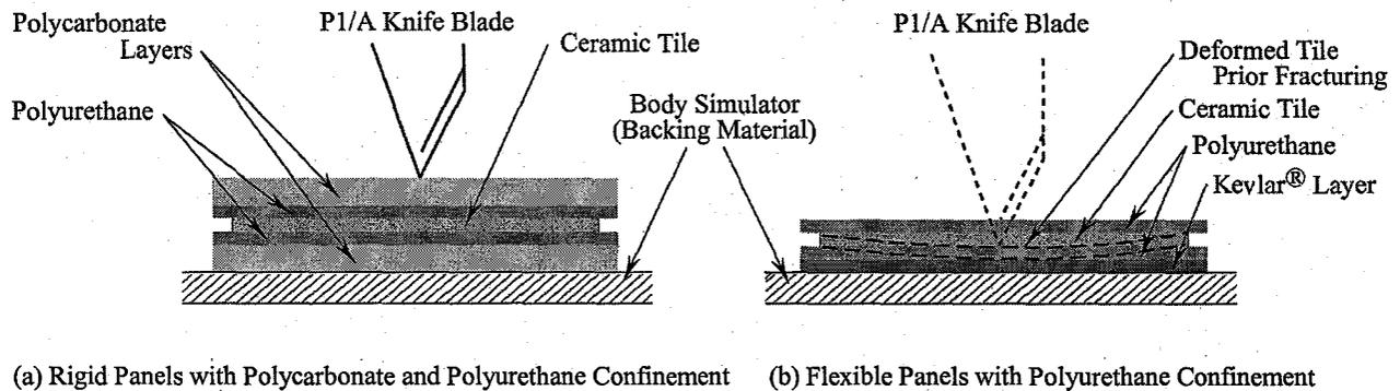
**Fig. 2** Support system with and without polycarbonate confinement
