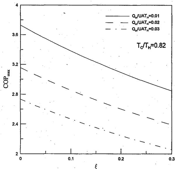
Fig. 4 Optimal coefficient of performance for typical freezing system.
