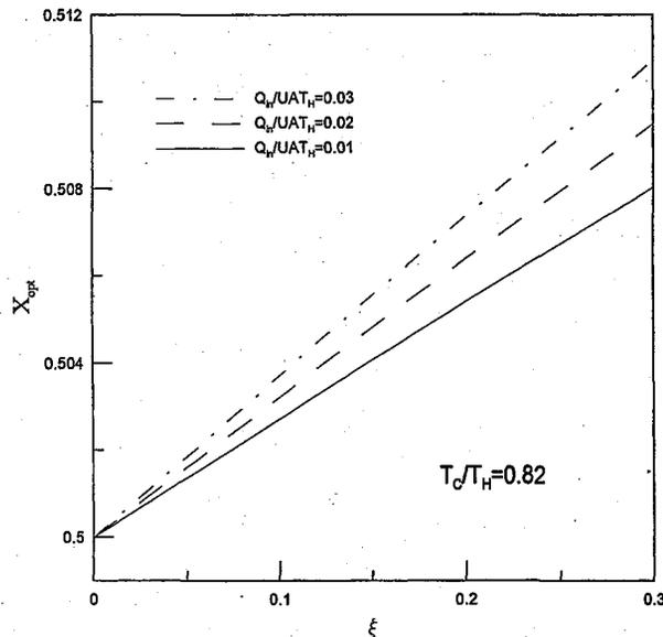
Fig. 2 Optimal allocation of thermal conductance for typical freezing system.
