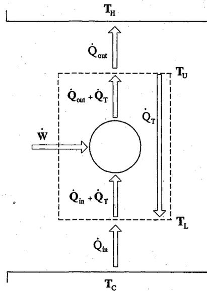
Fig. 1 Model of realistic refrigeration plant
