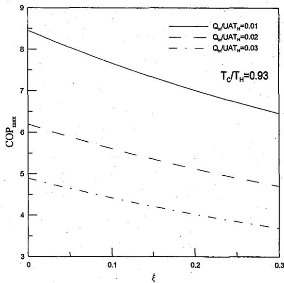
Fig. 5 Optimal coefficient of performance for typical air-conditioning system.
