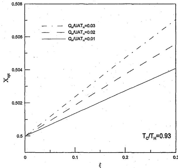
Fig. 3 Optimal allocation of thermal conductance for typical air-conditioning system.
