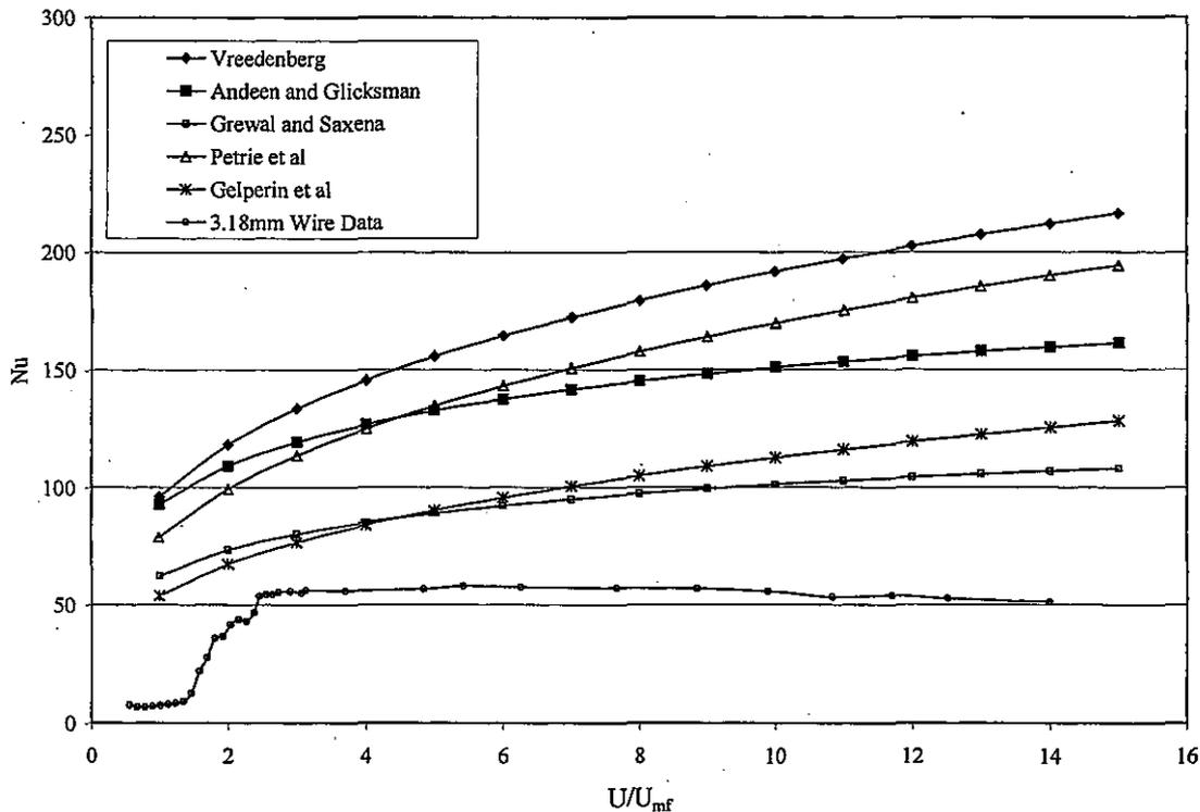
**Figure 1:** Comparison of standard correlations to data for heat transfer to a 3.18mm wire in a fluidized bed (from [2])
