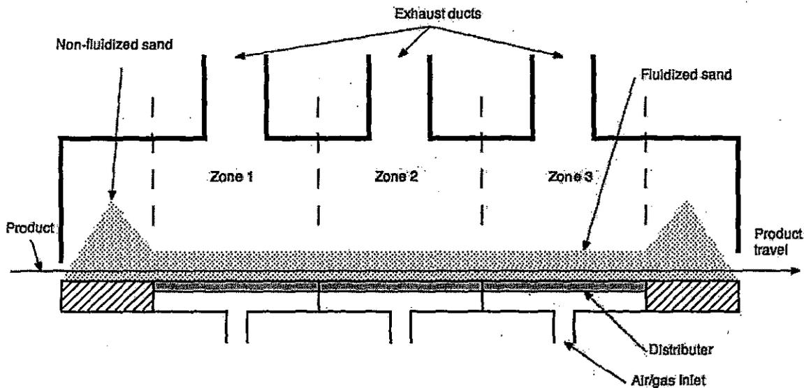
**Figure 2:** Schematic cross-section of a typical fluidized bed heat treating furnace.
