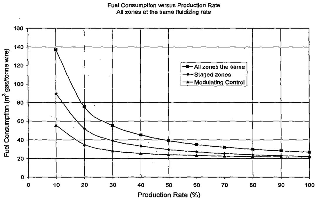
**Figure 3:** Fuel usage versus furnace loading using three different control schemes
