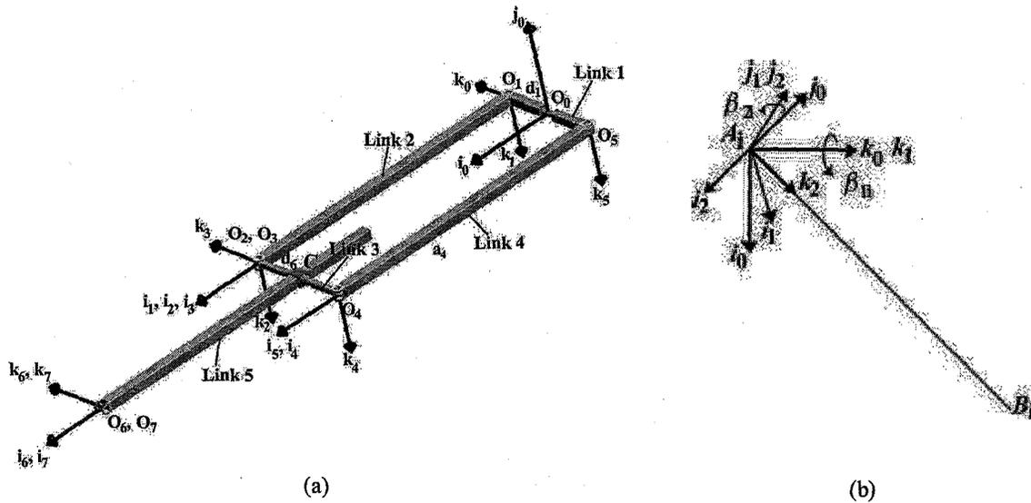
Figure 3 (a) Zero configuration of the rigid branch, (b) Rotating frames attached to a wire at the base.
