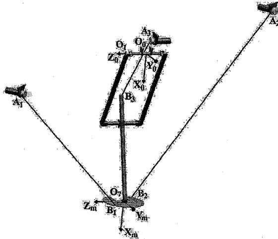
Figure 1 Considered 4 degrees of freedom wire-actuated parallel manipulator.
