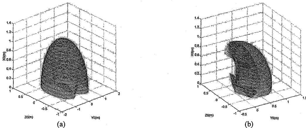
Figure 4 Workspace of the wire-actuated parallel manipulator (a) simulated one (b) prototyped one.
