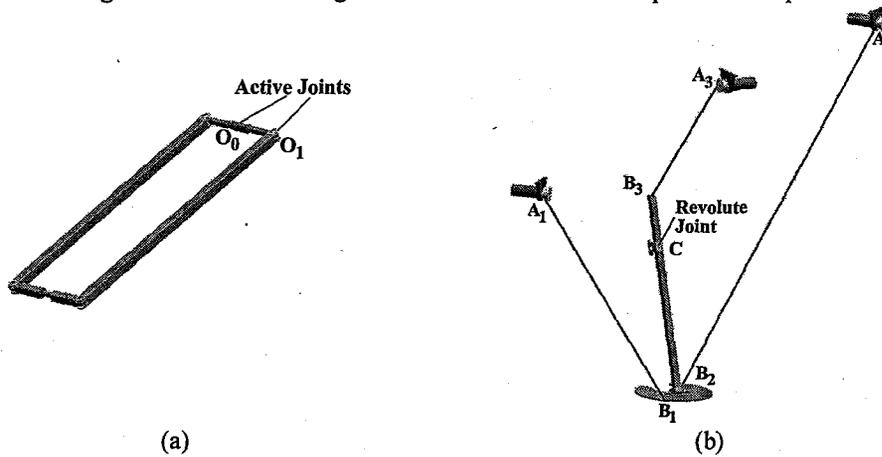
Figure 2 (a) Parallelogram mechanism, (b) Serial mechanism of the wire-actuated parallel manipulator.
