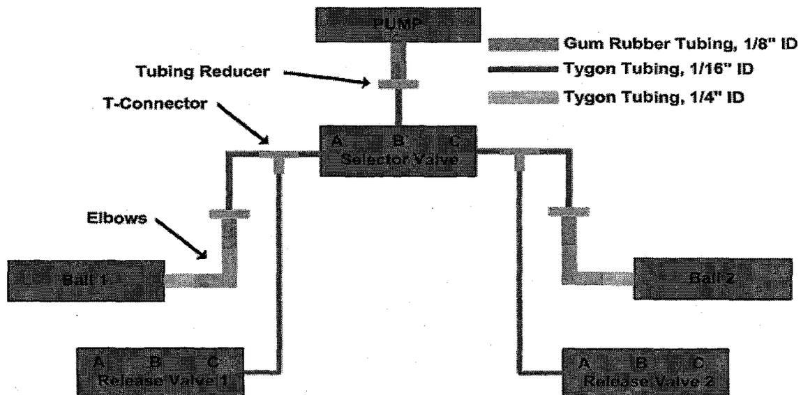
**Figure 3** – Schematic representation of the connections between the pump, the valves and the wheels.
