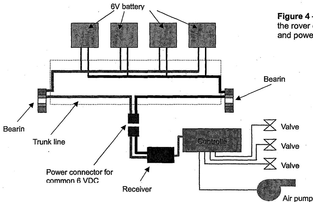
Figure 4 – Diagram of the rover control system and power transmission
