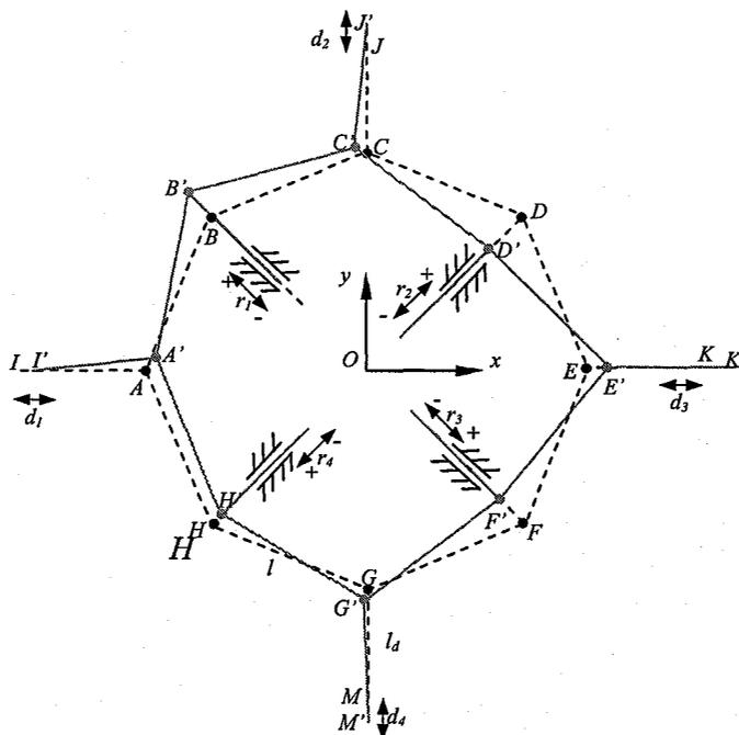
Figure 6. Kinematic model of the stimulator.
