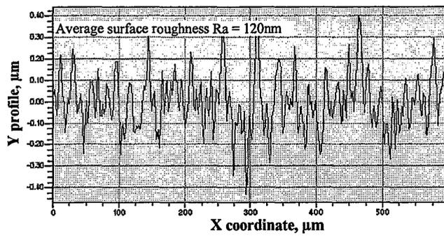
Figure 4. Machined PMMA surface roughness.
