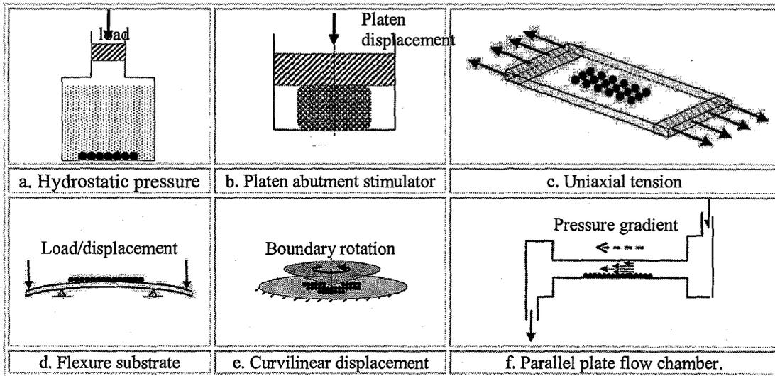
Figure 1. Schematic diagrams of several state-of-the-art mechanical stimulators [10].
