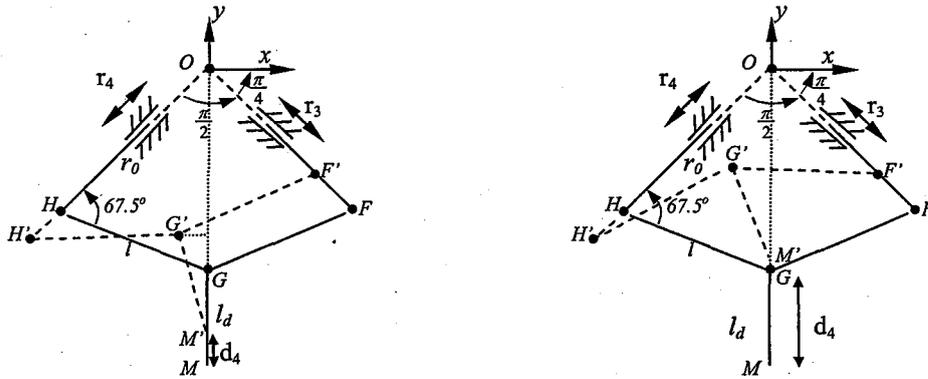
(a) The 1<sup>st</sup> inverse kinematic solution, (b) the 2<sup>nd</sup> inverse kinematic solution
