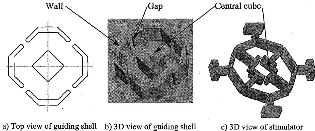
Figure 3. The layout of the stimulating mechanism and its guiding shell.
