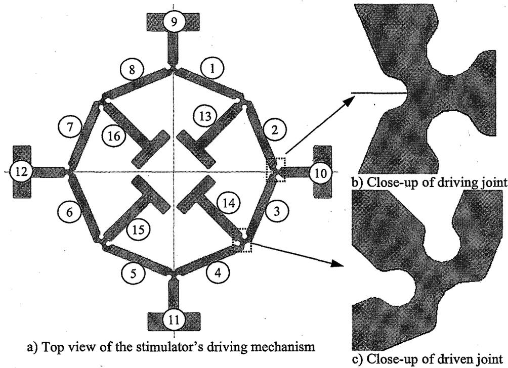
Figure 2. The 2D layout of the stimulator's driving mechanism.
