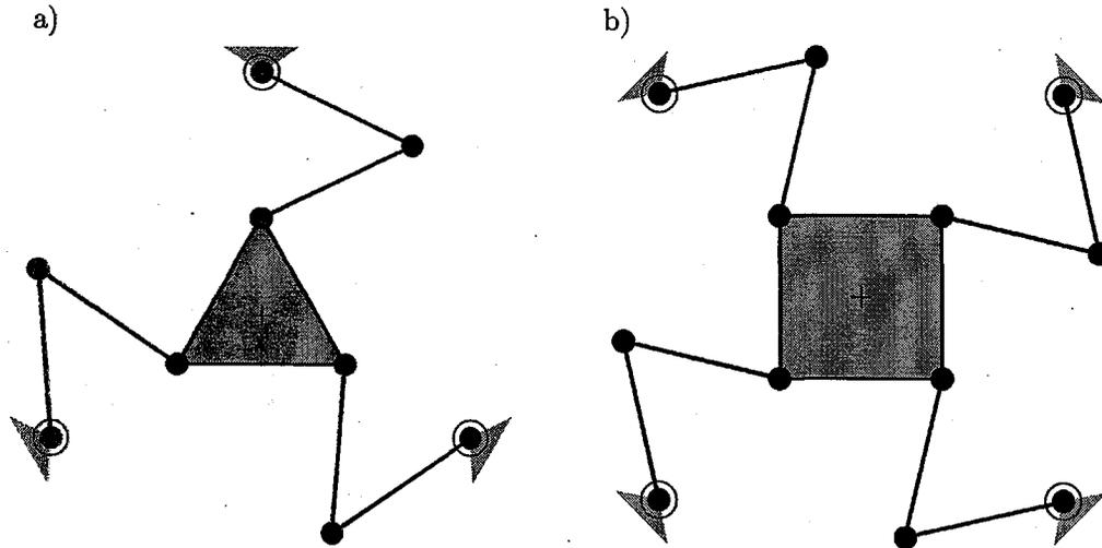
Figure 4: Planar Parallel Manipulators with Revolute Joints.
