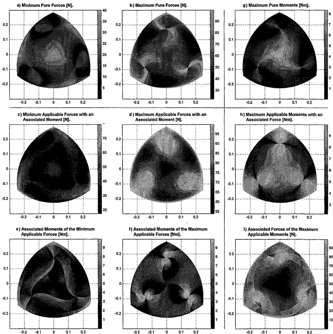
Figure 2: Force-Moment Capabilities of the 3-RRR PPM Throughout its Workspace. The X and Y Axes Define the Workspace [m] and the Greyscale Represents either Forces [N] or Moments [Nm].
