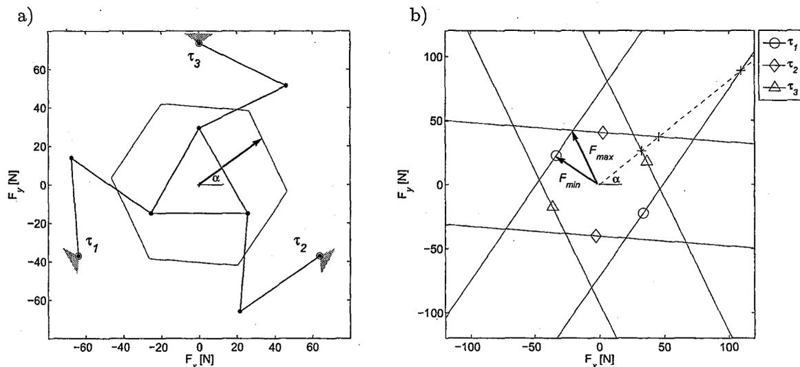
Figure 1: Generation of a Force Capability Polygon.
