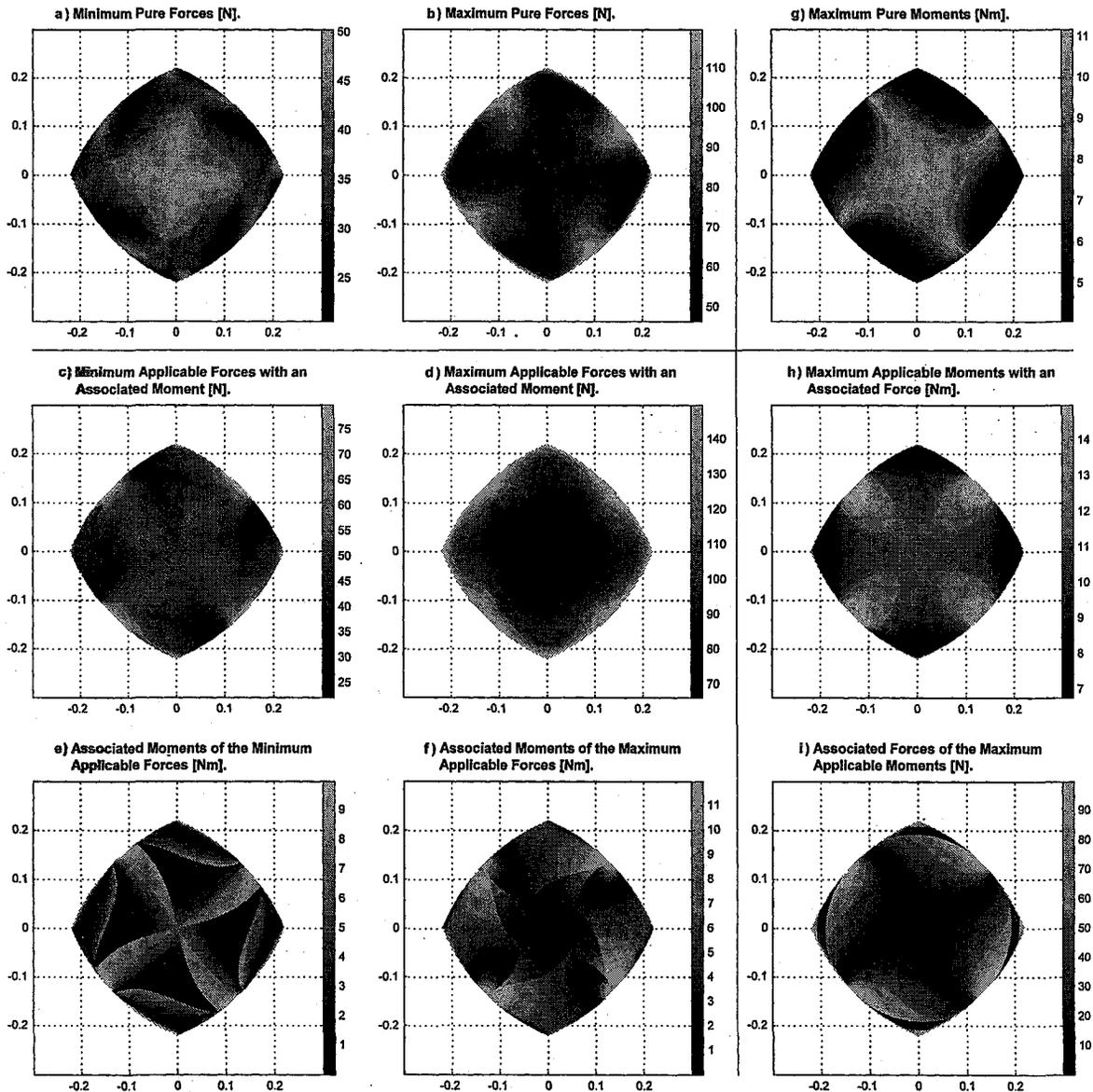
Figure 3: Force-Moment Capabilities of the 4-RRR PPM Throughout its Workspace. The X and Y Axes Define the Workspace [m] and the Greyscale Represents either Forces [N] or Moments [Nm].
