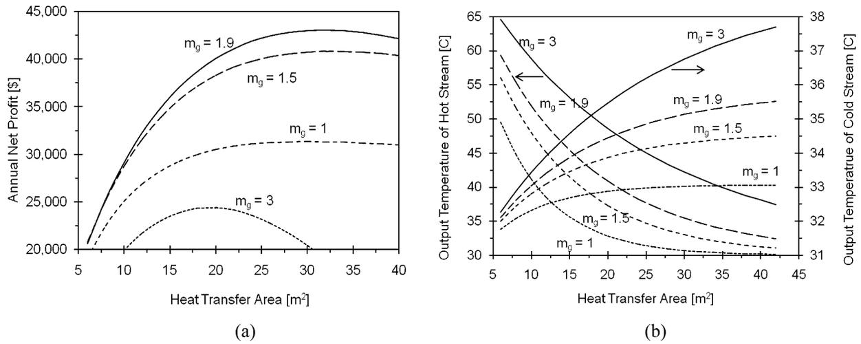
Fig. 3. (a) Annual profit and (b) outlet temperatures for a 1.5 inch pipe diameter
