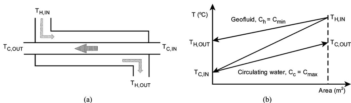
Fig. 1. (a) Schematic and (b) temperature profiles of a counter-flow heat exchanger
