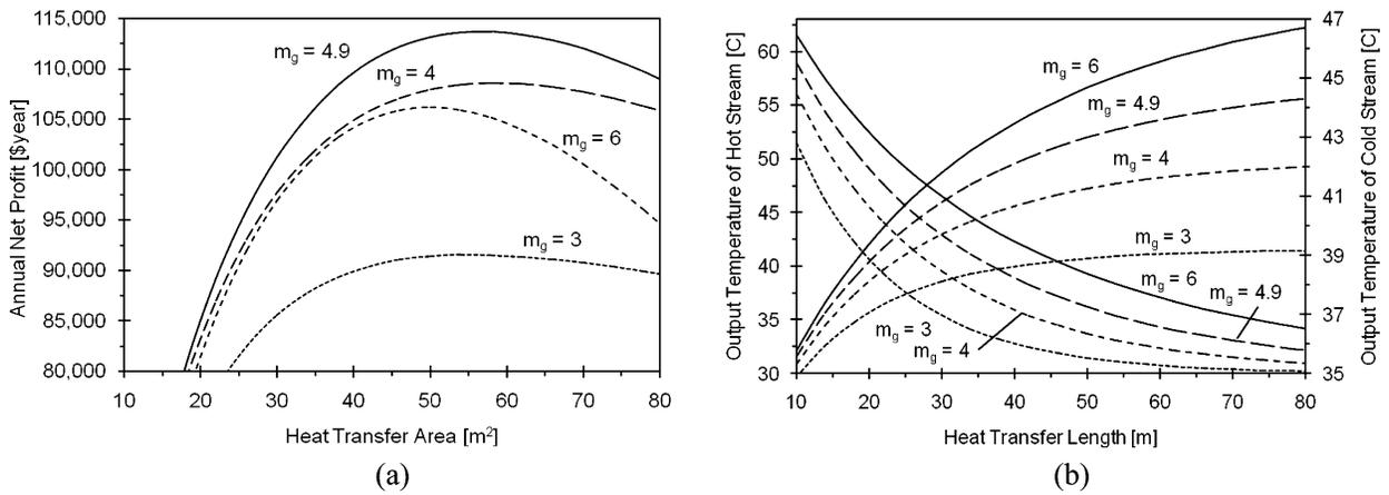
Fig. 4. (a) Annual profit and (b) outlet temperatures for a 2.5 inch pipe diameter
