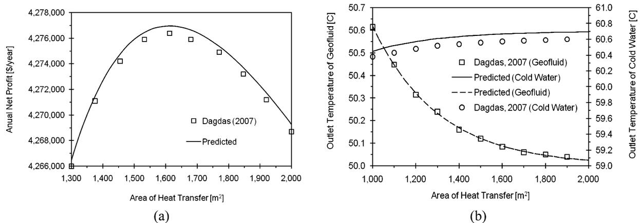
Fig. 2. (a) Annual net profit (Dagdas 2007) and (b) outlet temperatures of the geofluid and cold water
