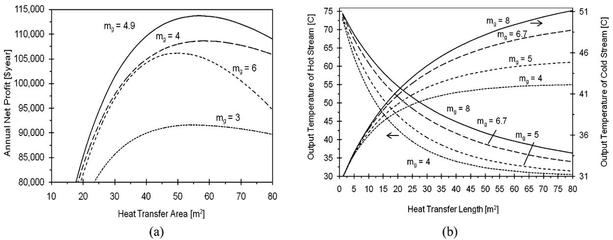
Fig. 5. (a) Annual profit and (b) outlet temperatures for a 3 inch pipe diameter
