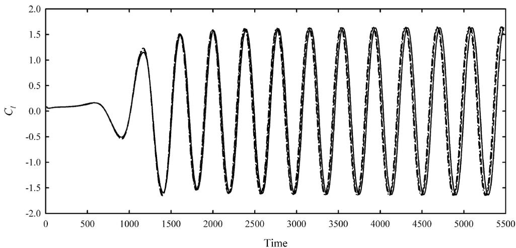
Fig. 3. Effects of near cylinder surface mesh sizes on the computations. — :  $\epsilon = 0.0026$ ; - - - - :  $\epsilon = 0.002$ ; - · - :  $\epsilon = 0.0016$ .
