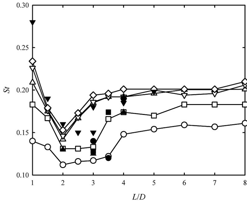
Fig. 5. Effects of  $Re$  and  $L/D$  on  $St$  in the cylinder wakes.  $\circ$  :  $Re = 100$ ;  $\square$  :  $Re = 200$ ;  $\triangle$  :  $Re = 500$ ;  $\nabla$  :  $Re = 800$ ;  $\diamond$  :  $Re = 1000$ ;  $\bullet$  : Slaouti and Stansby [8];  $\blacksquare$  : Papaioannou et al. [13];  $\blacktriangle$  : Meneghini et al. [7];  $\blacktriangledown$  : Igarashi [4] ( $Re = 2.2 \times 10^4$ ).
