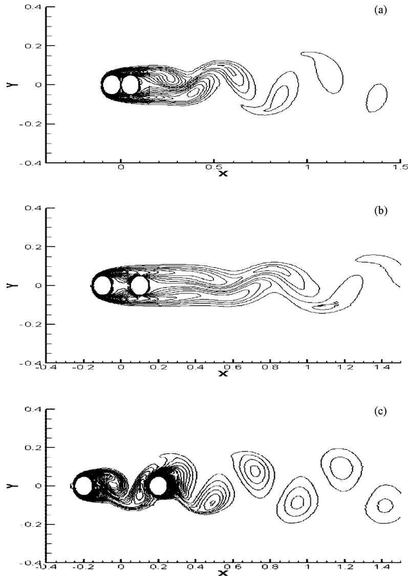
Fig. 4. Vorticity developments around the cylinders at  $Re = 200$ . (a)  $L/D = 1$ ; (b)  $L/D = 2$ ; (c)  $L/D = 4$ .
