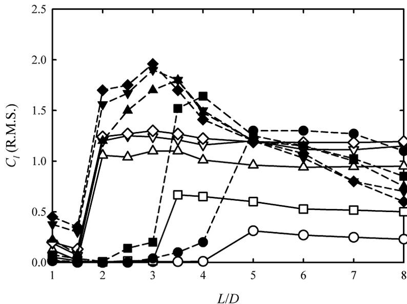
Fig. 6. Effects of  $Re$  and  $L/D$  on the  $C_l$  magnitudes.  $\circ$  :  $Re = 100$ ;  $\square$  :  $Re = 200$ ;  $\triangle$  :  $Re = 500$ ;  $\nabla$  :  $Re = 800$ ;  $\diamond$  :  $Re = 1000$ ; open symbol : upstream cylinder; closed symbol : downstream cylinder.
