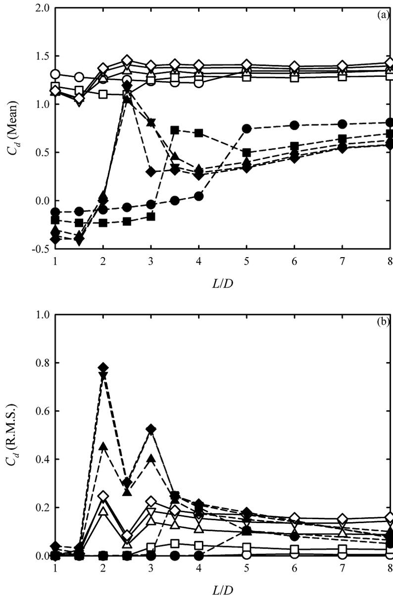
Fig. 8. Effects of  $Re$  and  $L/D$  on the  $C_d$  of the cylinders. (a) Mean  $C_d$ ; (b) Root-mean-square of  $C_d$  fluctuation. Legends : same as those for Fig. 6.
