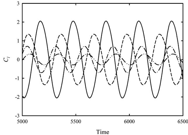
Fig. 7. Examples of lift fluctuations. — :  $Re = 500$ ,  $L/D = 4$  (Downstream cylinder); - - - - :  $Re = 500$ ,  $L/D = 4$  (Upstream cylinder); - · - :  $Re = 1000$ ,  $L/D = 1$  (Downstream cylinder); - · · - :  $Re = 1000$ ,  $L/D = 1$  (Upstream cylinder).
