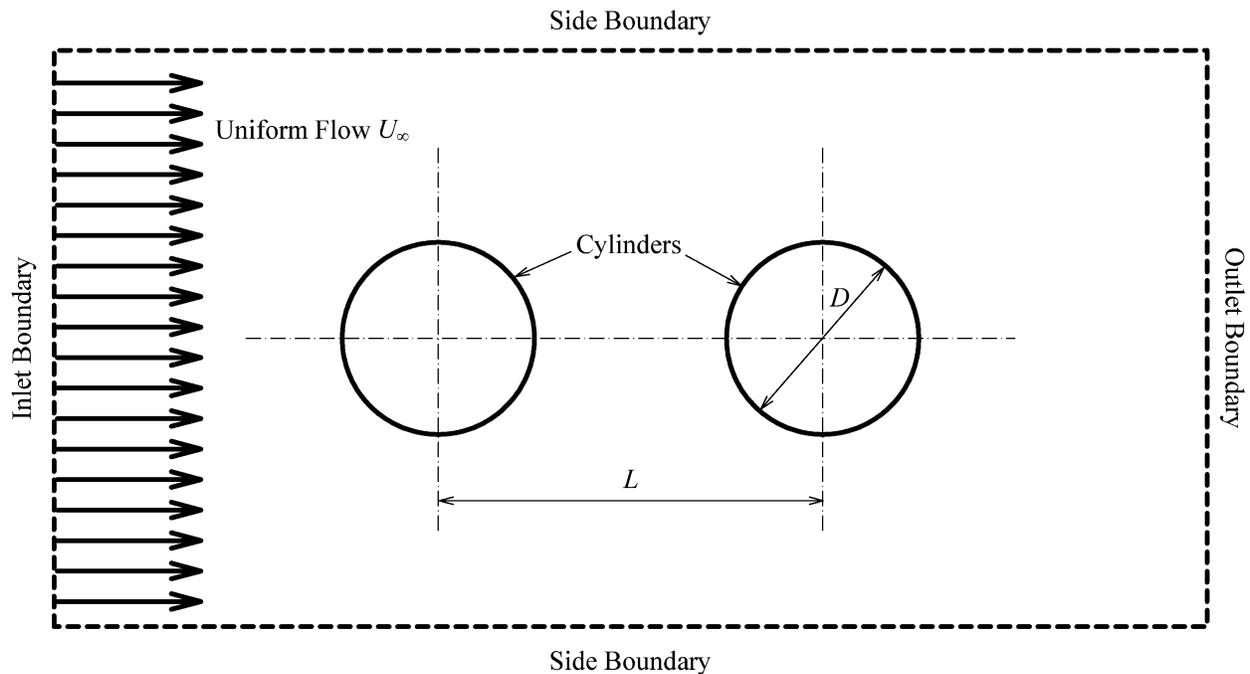
Fig. 1. Schematic for the tandem cylinder computational domain.
