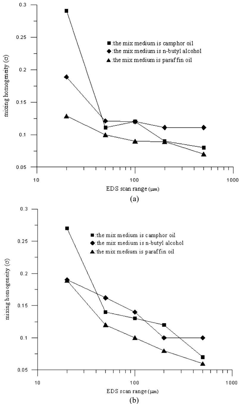
Fig. 7. The influence of mixing media on the mixing homogeneity for 3 vol.% 1  $\mu\text{m}$  W-Cu powders. (a) Powders fabricated in the TURBULA® mixer. (b) Powders fabricated in the Random mixer.
