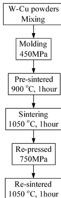
Fig. 3. Process schedule, including sintering, for W-Cu composite samples.
