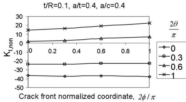
Fig. 7. Variations of  $K_{I,non}$  along the crack front for various crack positions  $\theta$ .
