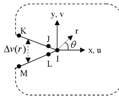
Fig. 5. Local Cartesian coordinates on crack tip.
