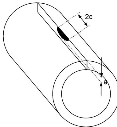
Fig. 2. A 3-dimensional semi-elliptical external crack.
