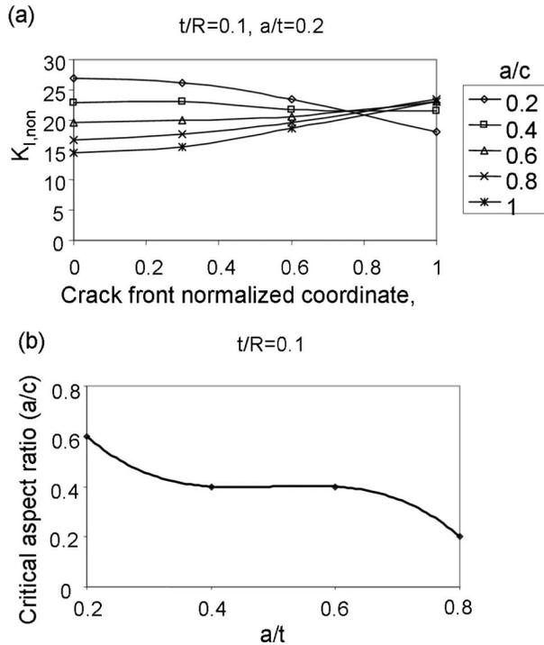
Fig. 10. Effect of crack aspect ratio  $a/c$  on mode I SIF for an external semi-elliptical crack in a buried pipe, a) Mode I SIF distribution along the crack front, b) critical ( $a/c$ ) at which maximum SIF transition takes place as a function of ( $a/t$ ).
