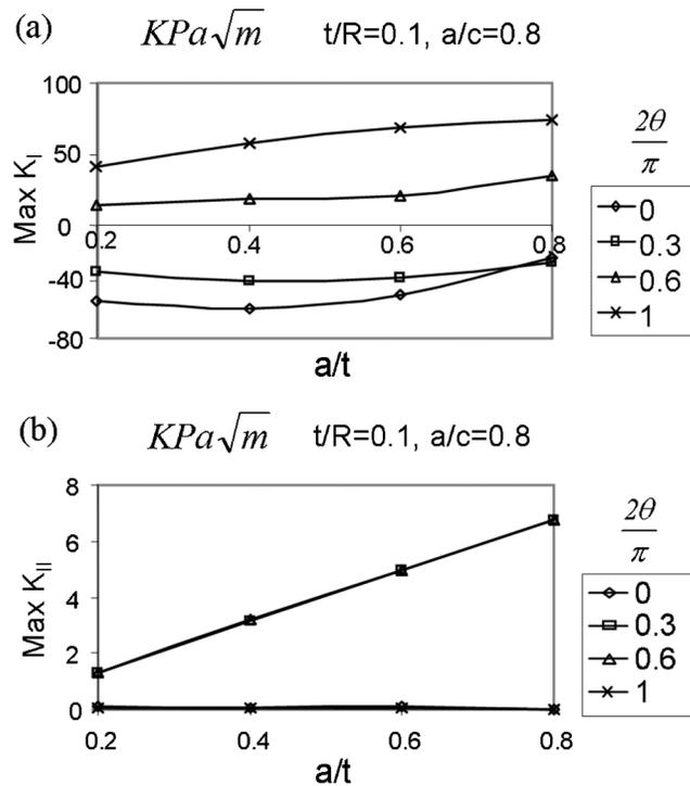
Fig. 9. Effect of relative crack depth ( $a/t$ ) on SIFs of an external semi-elliptical crack in, a) mode I, b) mode II.
