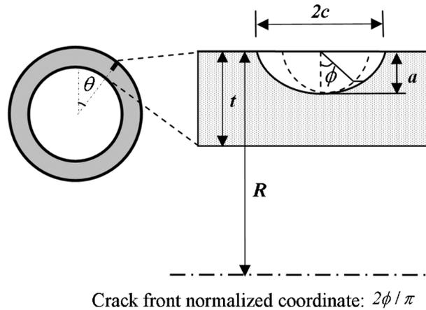
Fig. 3. Geometry of the pipe with an external axial crack of semi-elliptical shape.
