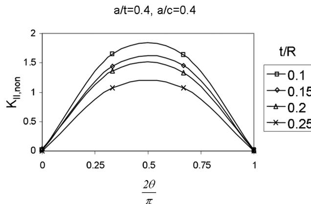
Fig. 6. Effect of crack orientation on  $K_{II}$  at deepest point for external semi-elliptical axial crack in buried pipe.
