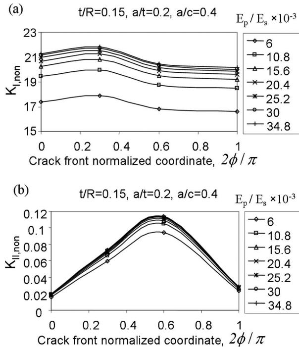
Fig. 11. Effect of  $E_p/E_s$  on stress intensity factors for an external semi-elliptical crack in a buried pipe, a) mode I, b) mode II.
