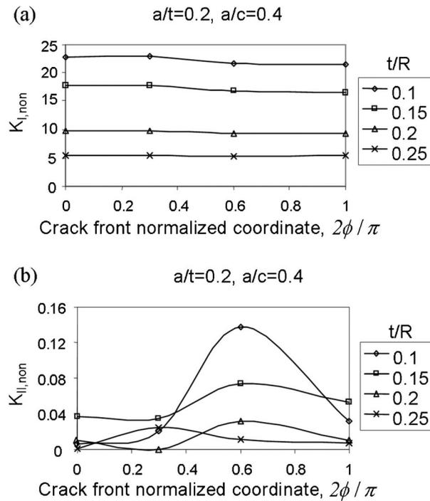
Fig. 8. Effect of relative wall thickness ( $t/R$ ) on SIFs of an external semi-elliptical crack, a) mode I, b) mode II.
