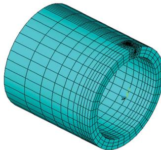
Fig. 4. Finite element model of pipe containing an axial crack.
