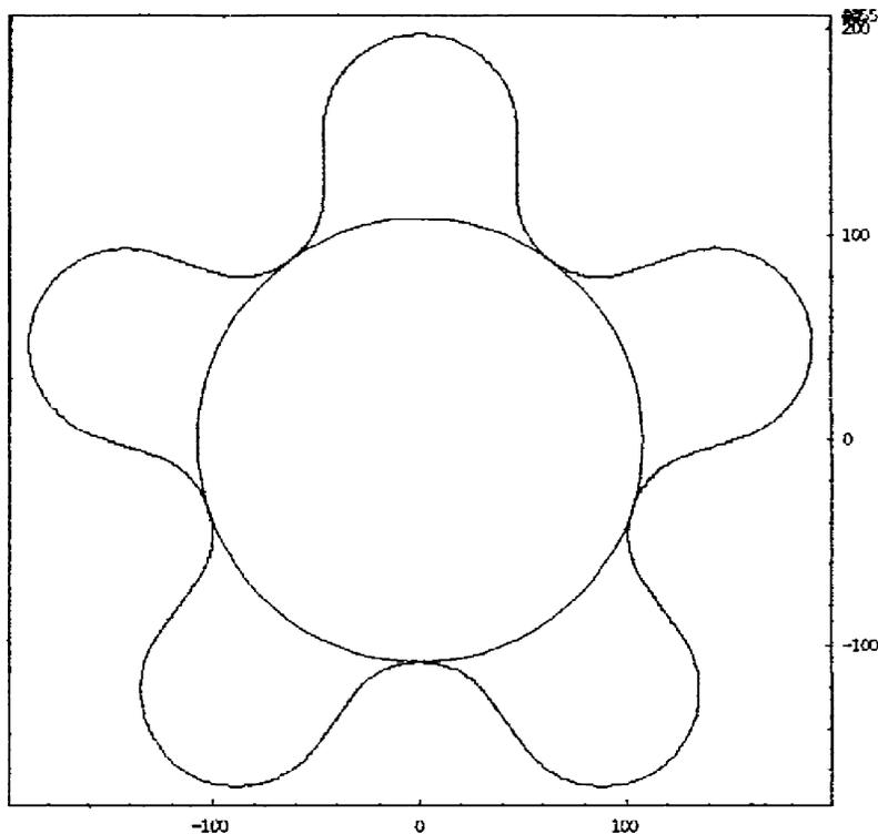
Fig. 4. The top land of the disc cutter was circular arc curve when  $w = 0$ .
