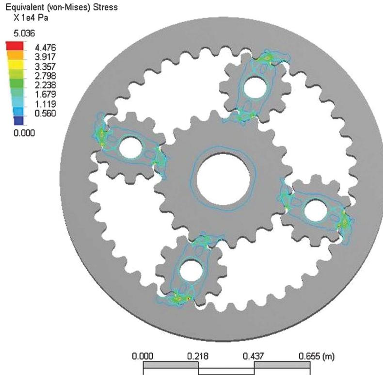
Fig. 7. The distribution of von-Mises stress for the proposed planetary gear mechanism (thickness=50mm,  $n_1=10$ ,  $\eta=1$ ,  $n_2=20$ ,  $n_3=40$ ,  $\alpha=\pi/36$ ,  $h=40$ ,  $r=108$ ,  $\theta_x=\frac{5\pi}{180\eta}$ ).
