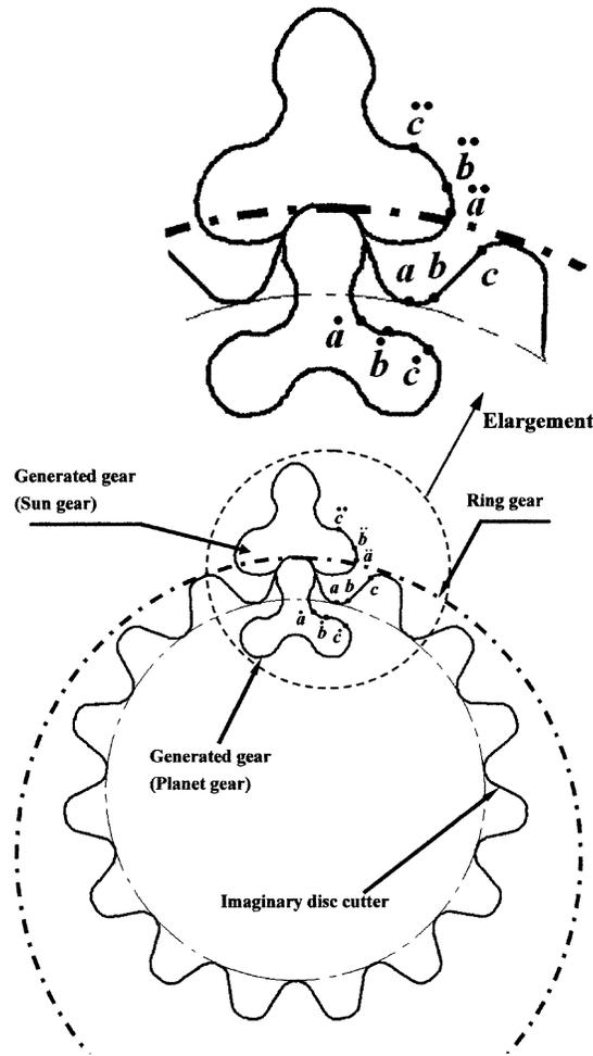
Fig. 1. The disc cutter composition with straight-line segment  $\overline{bc}$  and circular arcs  $\overline{ab}$  ( $\theta_x = \frac{\pi}{60\eta}$ ).
