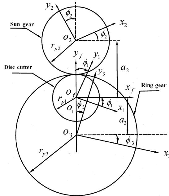
Fig. 5. The kinematics relationship among the sun gear, the ring gear and the disc cutter.
