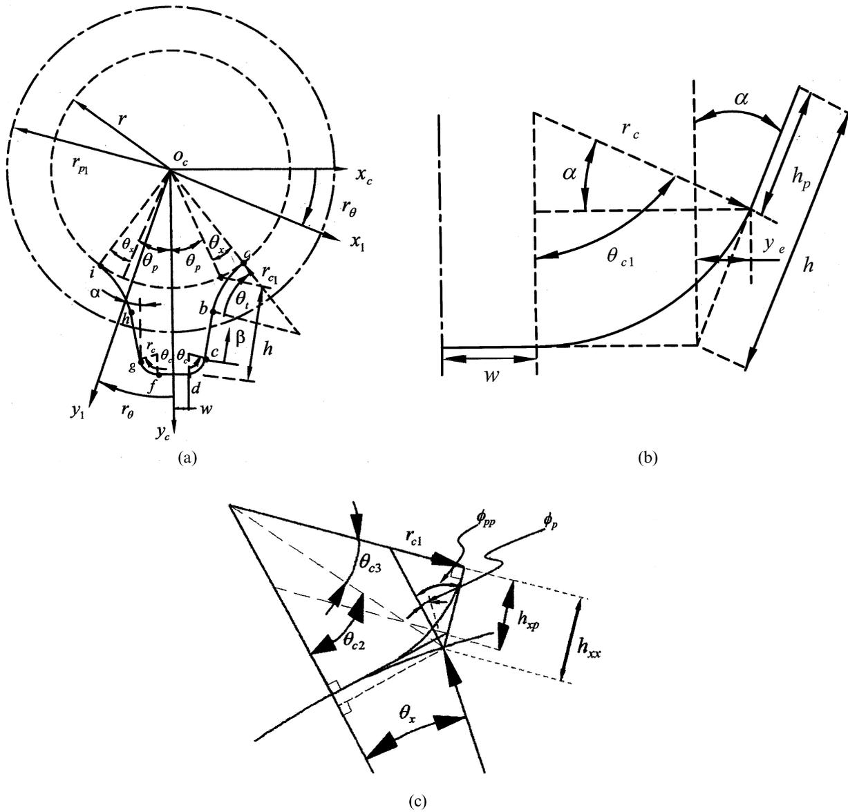
Fig. 3a. The proposed disc cutter design. 3b. The detail symbols on region  $\overline{cd}$ . 3c. The detail symbols on region  $\overline{ab}$ .
