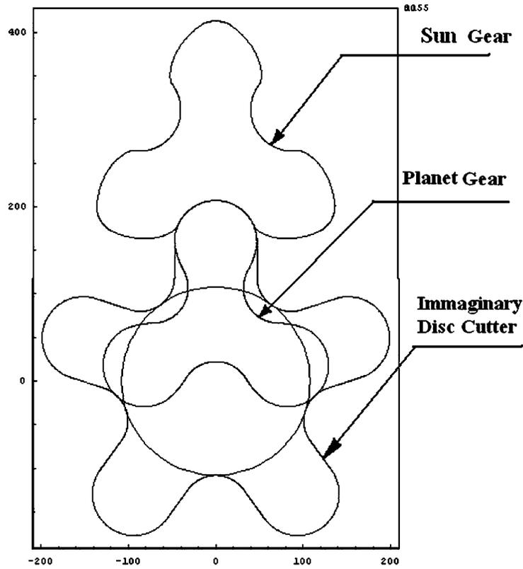
Fig. 6. The gear pump with small numbers of teeth generated by the imaginary disc cutter ( $\theta_x = \frac{10\pi}{180\eta}$ ).
