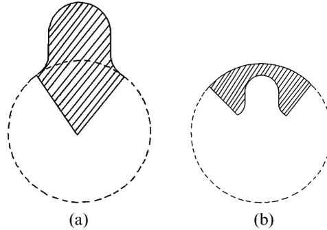
Fig. 2a. The imaginary disc cutter  $\Sigma_t$  is used to generate the sun gear. 2b. The imaginary disc cutter  $\Sigma_c$  is used to generate the planet gear.
