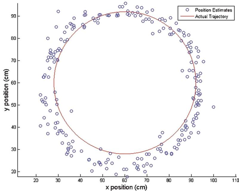
Fig. 12. Tracking test results for a beacon moving at 0.215 m/s around a circular track for a period of 60 s.
