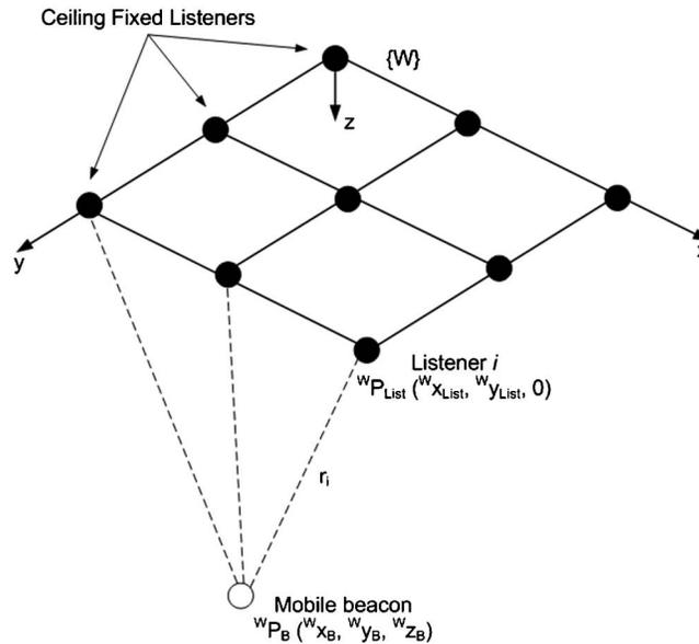
Fig. 4. Trilateration of the mobile beacon position.
