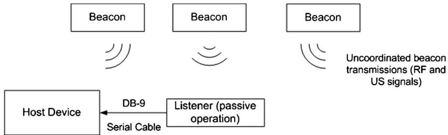
Fig. 2. Original cricket system architecture.
