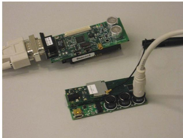
Fig. 6. Cricket node (top) and gumstix embedded controller (bottom) hardware.
