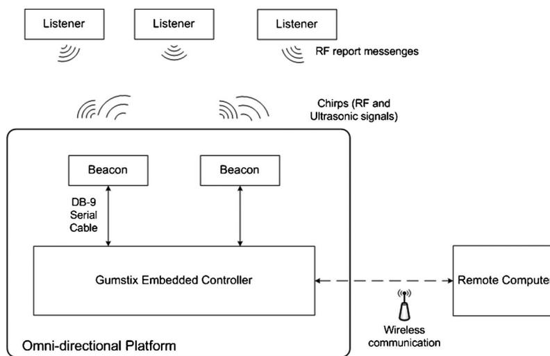
Fig. 3. Modified cricket localization system architecture.
