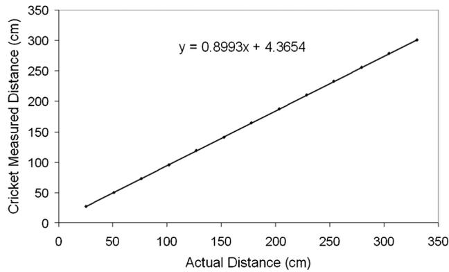
Fig. 10. Distance estimation test results.
