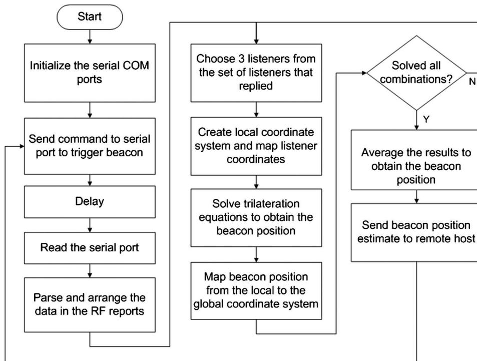
Fig. 9. Gumstix embedded controller program flowchart.
