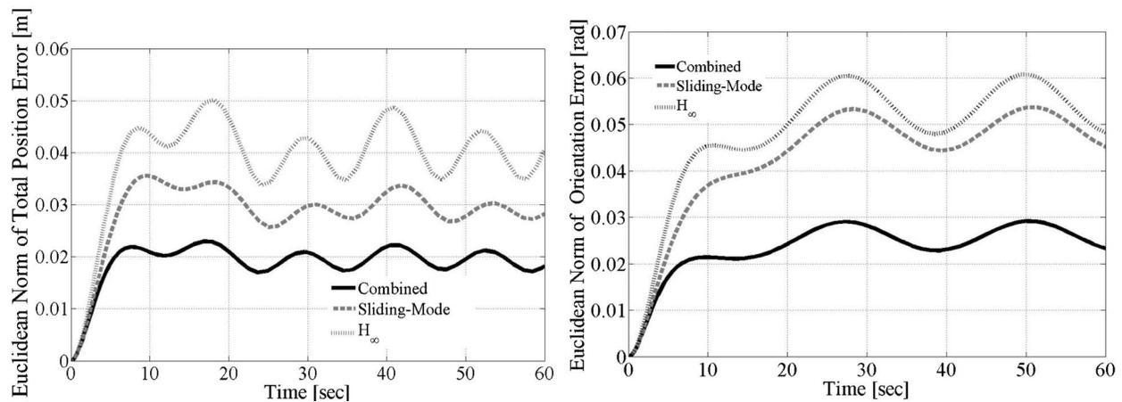
Fig. 10. Euclidean norm of position and orientation error for each controller. As can be seen from the figure that the combined  $H_\infty$ -Sliding-Mode controller outperforms the other two controllers.
