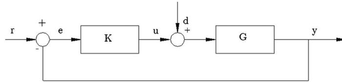
Fig. 2. Feedback control loop. The input disturbance force is given by d.
