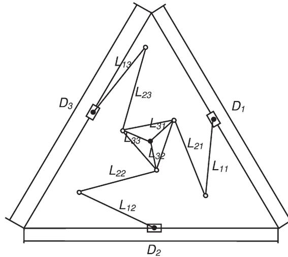
Fig. 1. Kinematically redundant 3-PRRR planar parallel manipulator [6].
