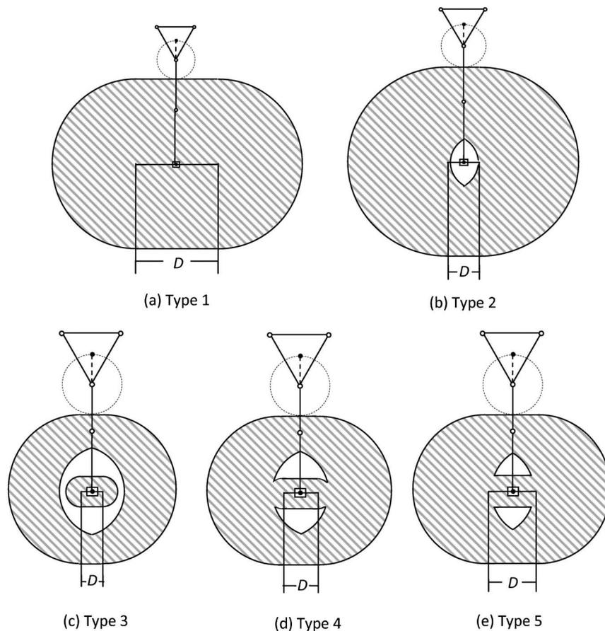
Fig. 6. Types of workspaces of the individual legs of a kinematically redundant planar parallel manipulator (PRRR).
