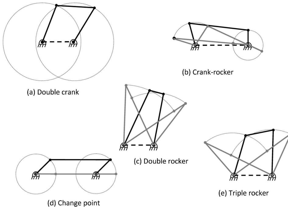
Fig. 3. Categories of four-bar mechanisms (adapted from [7]).
