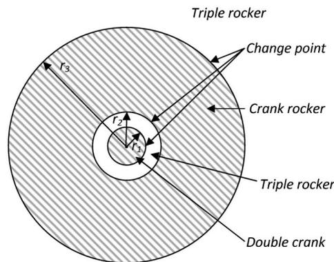
Fig. 5. Transition from one category of four-bar mechanisms to another.
