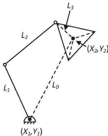
Fig. 2. One leg without the prismatic actuator (RRR).
