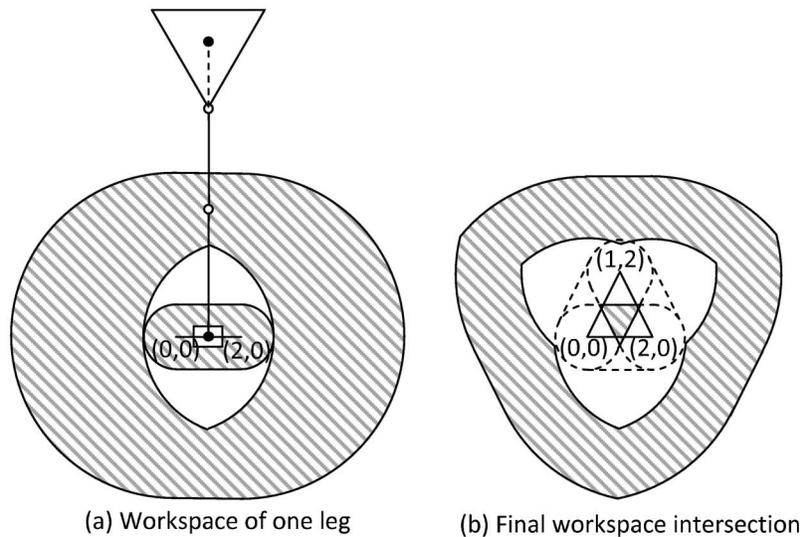
Fig. 8. Workspace of one of the PRRR legs and the final workspace of a 3-PRRR kinematically redundant planar parallel manipulator.
