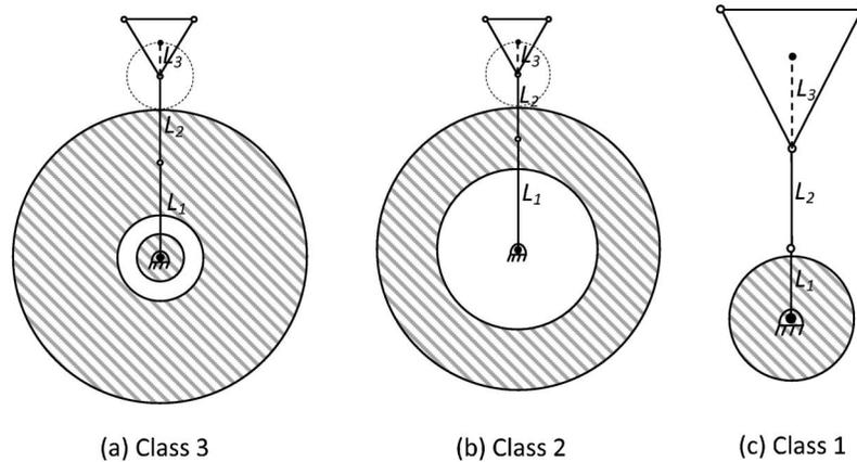
Fig. 4. Classes of the workspace of each leg without the influence of the prismatic actuator.
