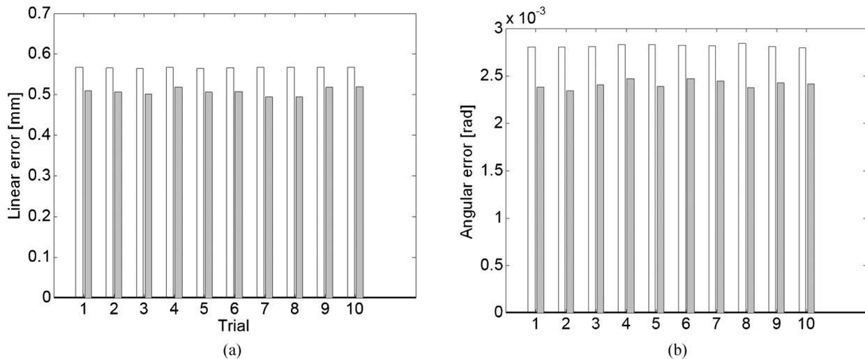
Fig. 5. Comparison, for 10 different trials, between the resolution of the actual ISL computed by applying differential transformation theory, Eqs. (16,b), (white bars), and the end-effector pose error computed numerically by adding randomly distributed uncertainties to the joint variables, Eqs. (18a,b), (grey bars). (a) Linear error and (b) angular error.
