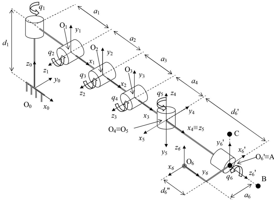
Fig. 2. Schematic view of the actual 6R-ISL with embedded frames and nominal geometrical parameters, in its reference configuration. Parameters  $d_6' = 100\text{mm}$  and  $d_6'' = -75\text{ mm}$ , to give  $d_6 = d_6' + d_6''$ , are used into the text. Points A, B and C are used to solve for the inverse kinematics.
