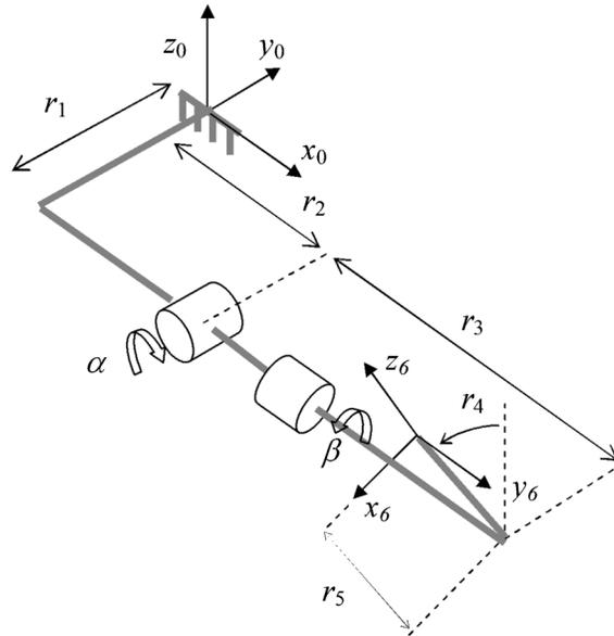
Fig. 4. Schematic representation of the ‘virtual joint’, i.e. the 2-DOF model of the knee articulation, used to estimate ISL kinematic performance. Geometric parameters  $r_1, \dots, r_5$  (whose values are given into the text) are used to define the ‘leg’, while angles  $\alpha, \beta$  represent the two degrees of freedom relative to the flexion-extension and longitudinal internal-external rotation, respectively.
