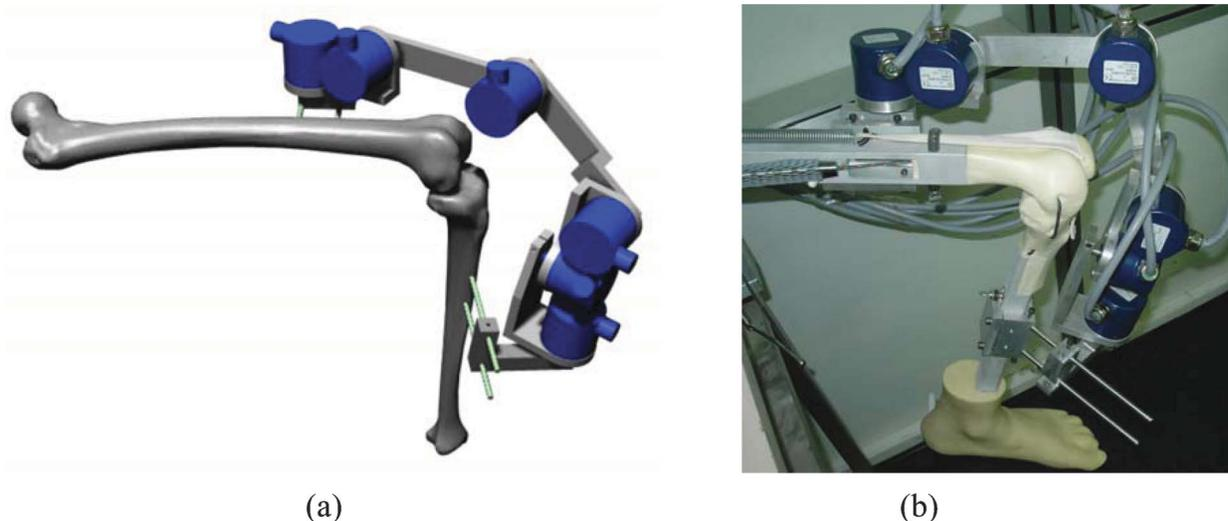
Fig. 1. The actual 6R-ISL. (a) Virtual representation (CAD models of tibia and femur were created by Marco Viceconti and are available on the Internet through the BEL Repository managed by the Istituti Ortopedici Rizzoli, Bologna, Italy). (b) Picture of the real system on a workshop leg system (MITA Endo Leg, Medical Models Ltd. UK).
