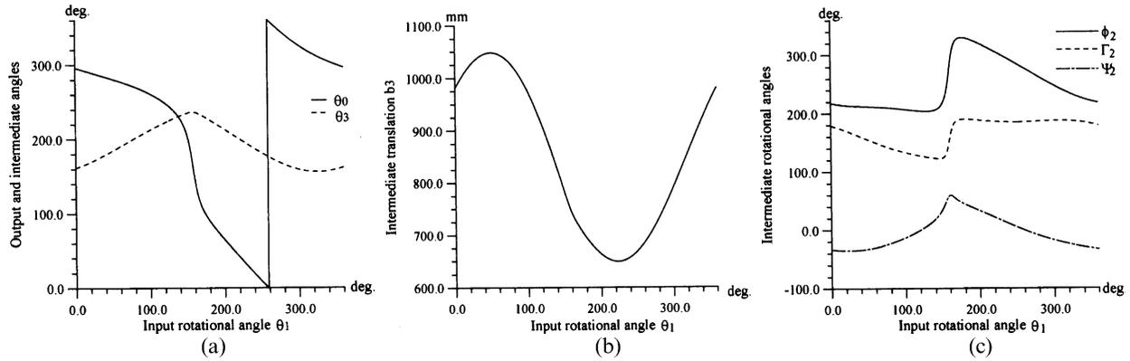
Fig. 6. Variation of intermediate displacements of RSCR mechanism.
