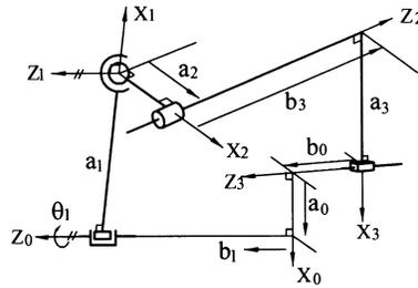
Fig. 8. Illustration of RSCP mechanism.
