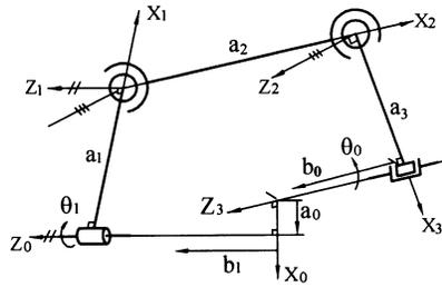
Fig. 12. Illustration of CSSR mechanism.
