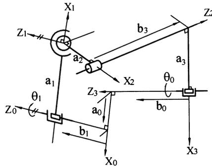
Fig. 5. Illustration of RSCR mechanism.
