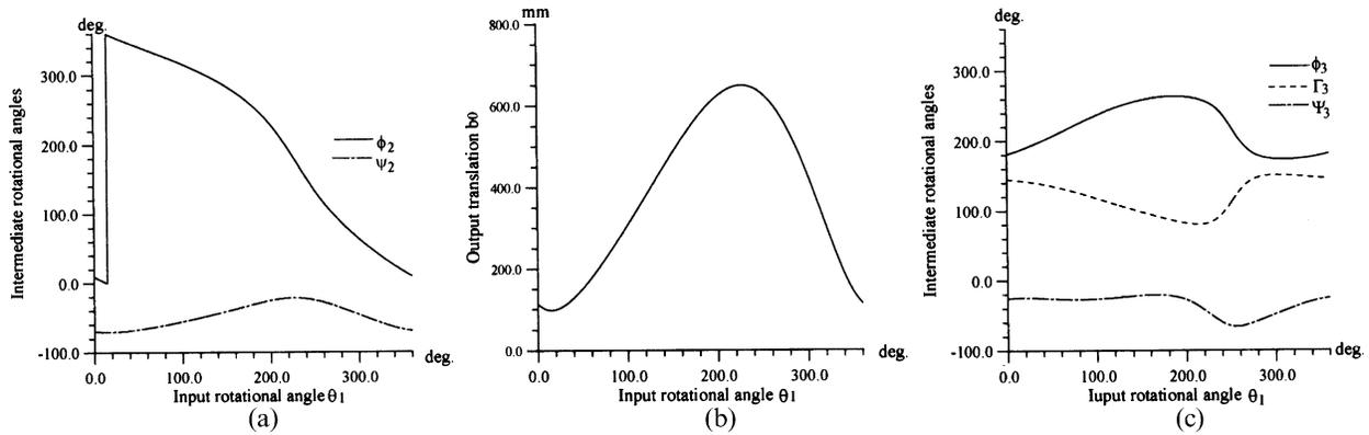
Fig. 10. Variation of intermediate displacements of CSSP mechanism.
