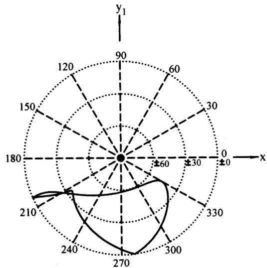
Fig. 7. Contour  $\Sigma_1$  traced by  $x_2$  axis of RSCR mechanism.
