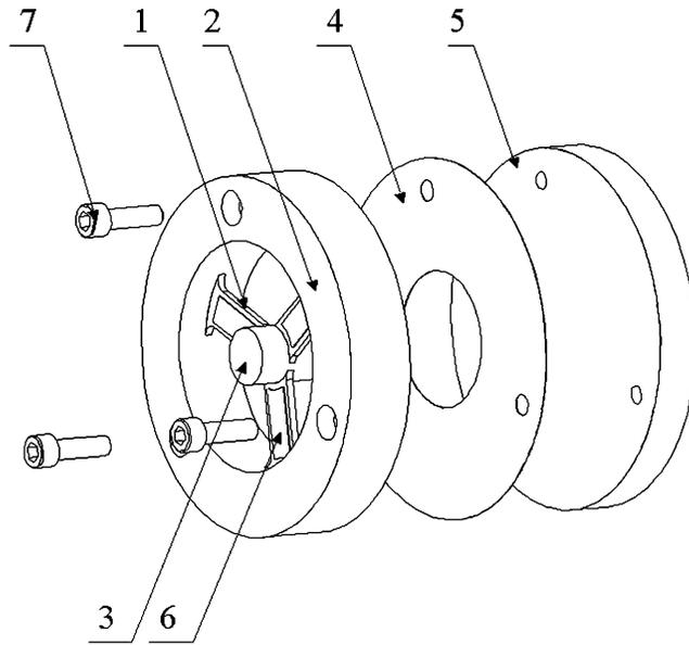
Fig. 1. The exploded view of the load cell: flexure beam (1); solid ring (2); hub (3); shim (4); solid disk (5); stain gauge (6); bolt (7).
