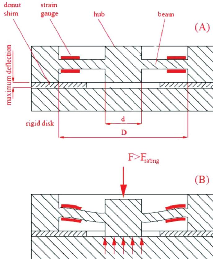
Fig. 2. The cross section view of the sensor: (A) no deflection, (B) maximum deflection.
