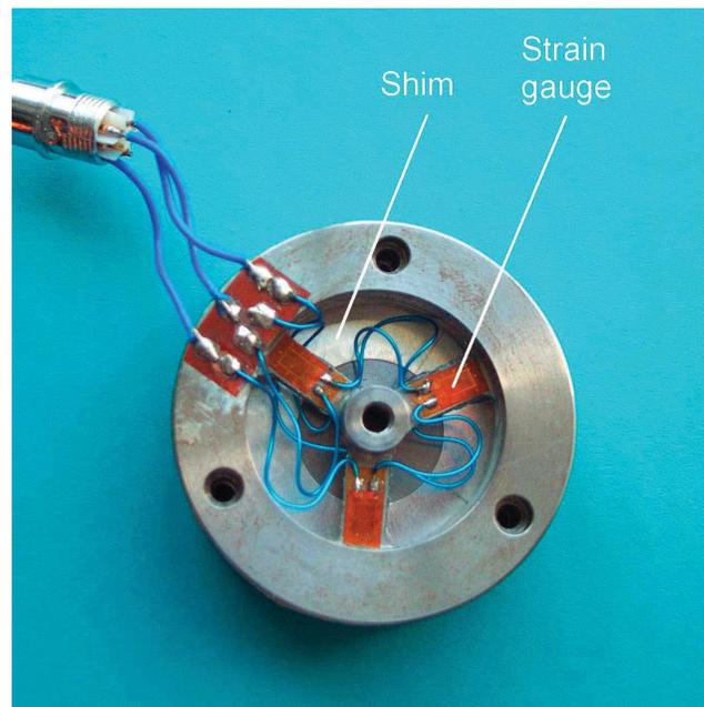
Fig. 5. The load cell prototype.
