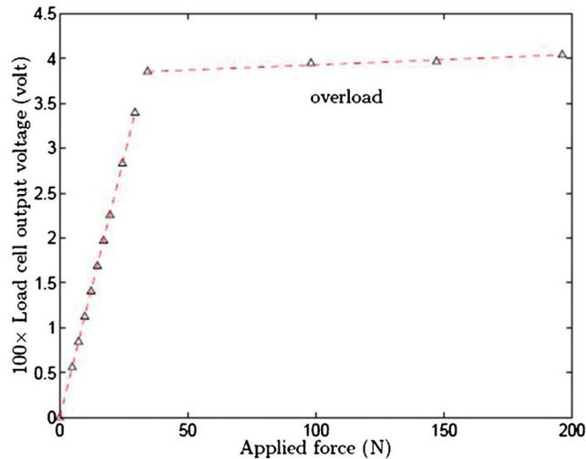
Fig. 7. Sensor output versus applied loads.
