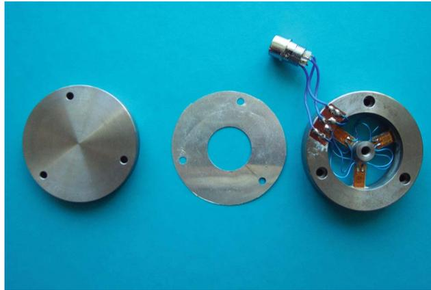
Fig. 6. The sensor components: body of sensor (A), shim (B), rigid disk (C).
