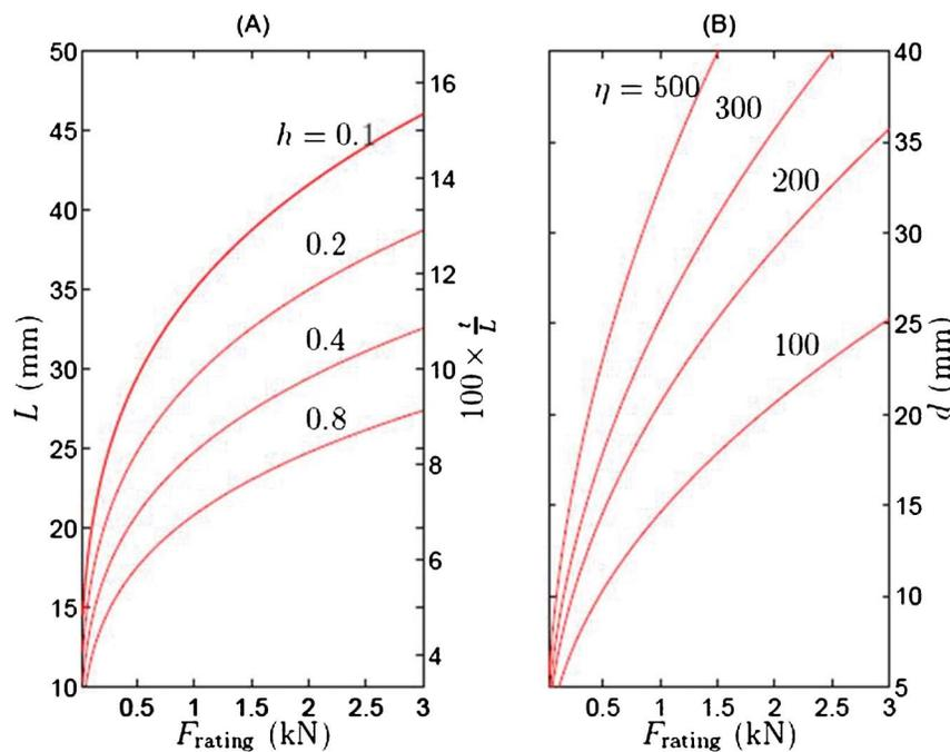
Fig. 4. The beam length (A) and hub diameter (B) versus different rating loads.
