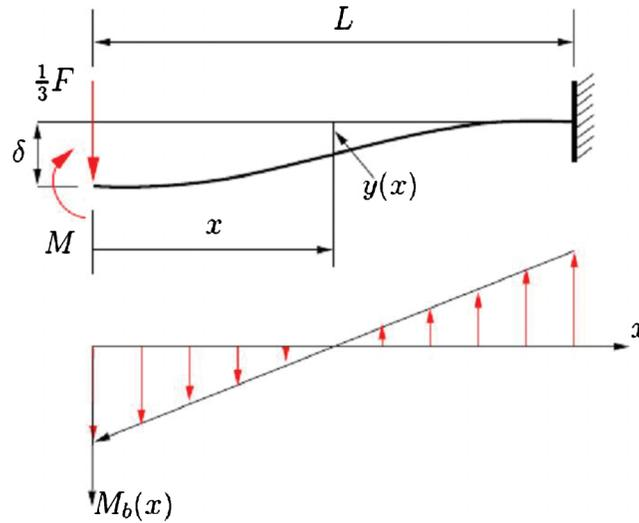
Fig. 3. One of the sensor's flexure.
