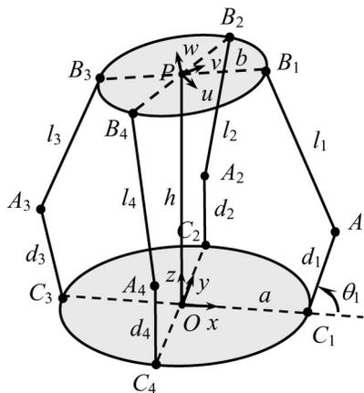
Fig. 3. The schematic model of a 4RUS+1PS parallel manipulator.
