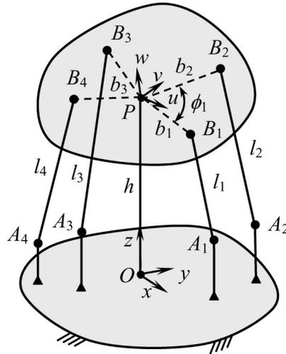
Fig. 2. The 4US+1PS structure.
