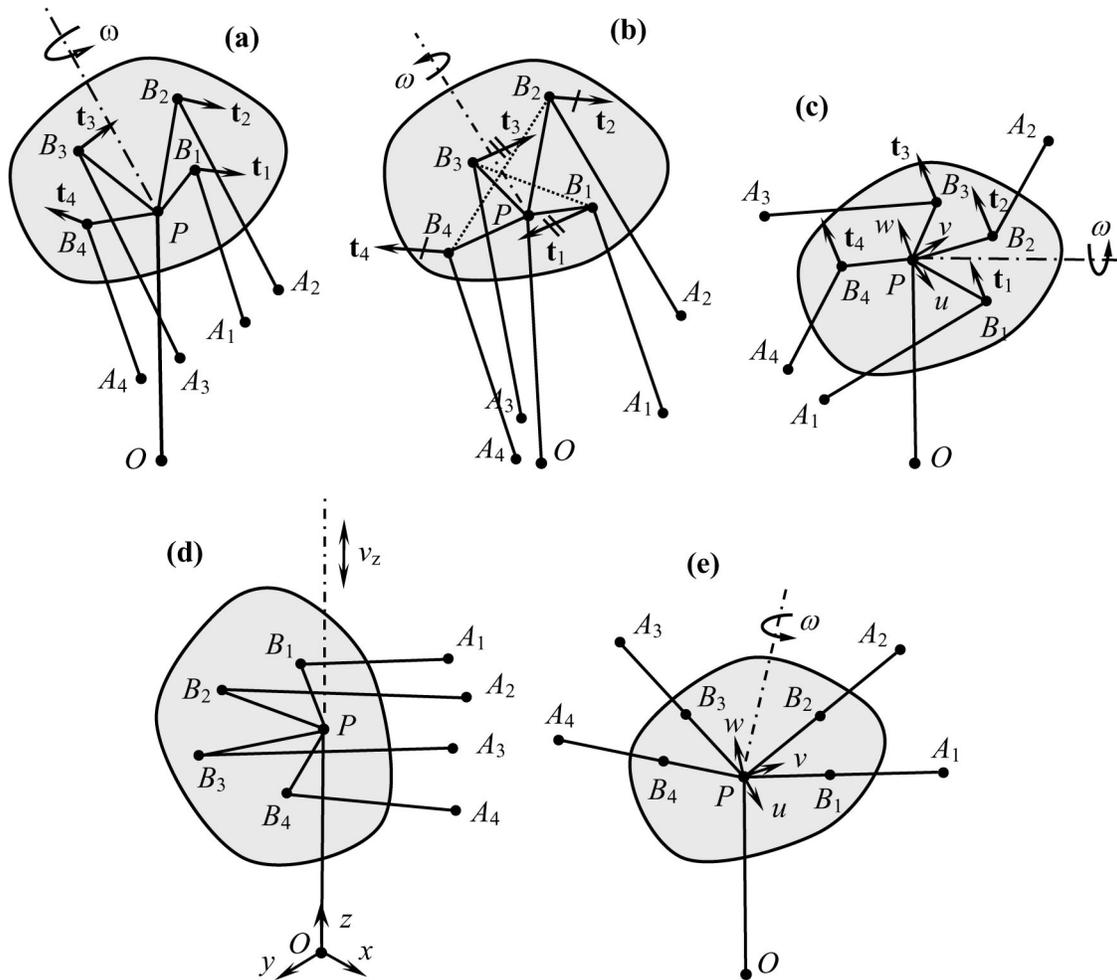
Fig. 6. Five cases of direct kinematic singularities of the manipulators: (a) when vectors  $\mathbf{t}_i$  are coplanar, (b) when vectors  $\mathbf{t}_i$  are parallel two by two, (c) when vectors  $\mathbf{t}_i$  are parallel with each other, (d) when vectors  $\mathbf{l}_i$  ( $i=1, \dots, 4$ ) are parallel with the  $xy$  plane and (e) when vectors  $\mathbf{t}_i$  are zero.
