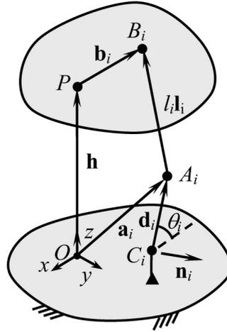
Fig. 5. Sketch of a typical leg of the 4-RUS+1PS parallel manipulator.
