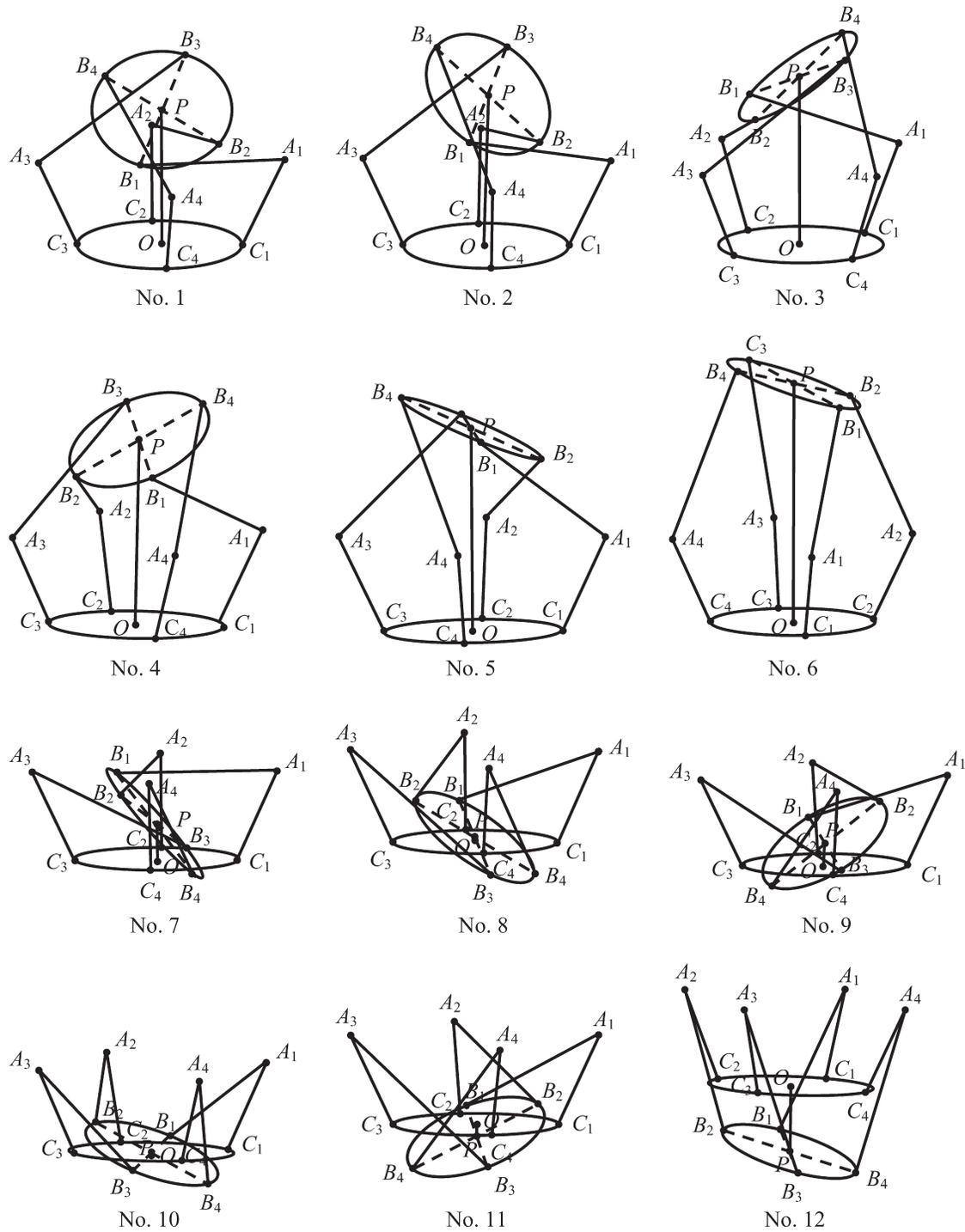
Fig. 4. Twelve solutions of the direct kinematics problem corresponding to assembly modes of the 4RUS+1PS manipulator.
