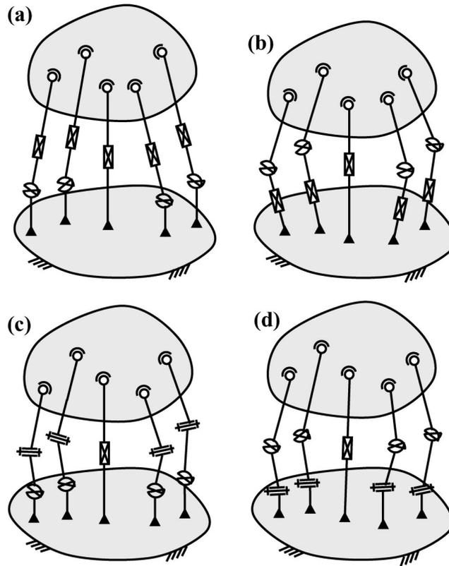
Fig. 1. Kinematic diagram of members of the family: (a) 4UPS+PS, (b) 4PUS+PS, (c) 4URS+PS (d) 4RUS+PS.
