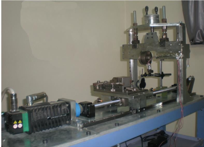
Fig. 3. Quick stop device.
