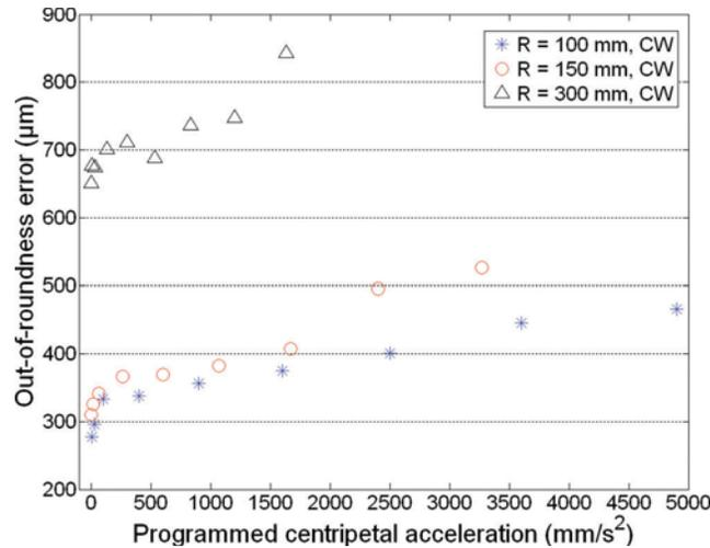
Fig. 9. Out-of-roundness as a function of programmed centripetal acceleration for a horizontal circular path of various radii centred at approximately  $\{-290 \text{ mm}, 987 \text{ mm}, 615 \text{ mm}\}$ .
