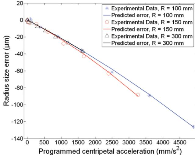
Fig. 10. Experimental and predicted radius size error as a function of the programmed centripetal acceleration for a horizontal circular path of various radii centred at approximately  $\{-290 \text{ mm}, 987 \text{ mm}, 615 \text{ mm}\}$ .
