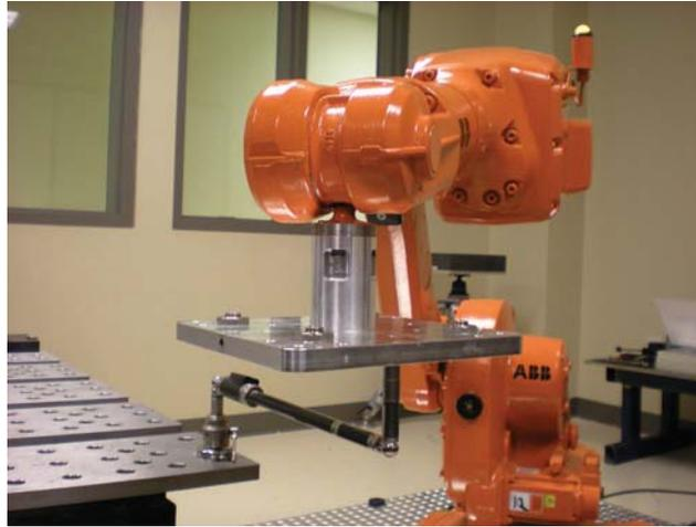
Fig. 1. Telescoping ballbar setup for measuring radial errors along a horizontal circular path of radius 300 mm.
