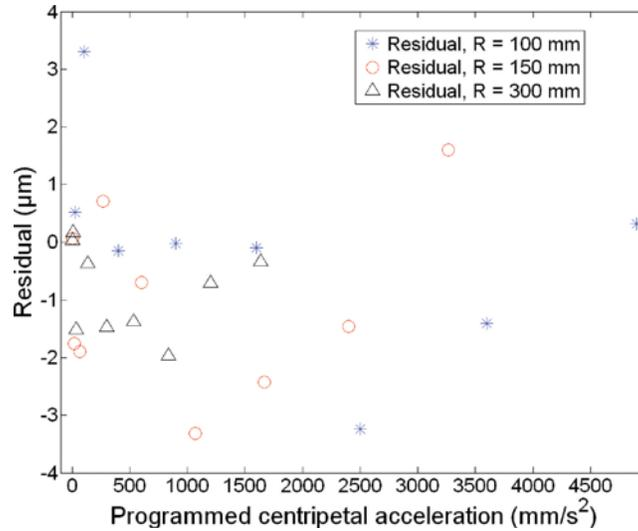
Fig. 11. Residuals between the experimental and predicted radius size error as a function of programmed centripetal acceleration for horizontal circular paths of various radii centred at approximately  $\{-290 \text{ mm}, 987 \text{ mm}, 615 \text{ mm}\}$ .
