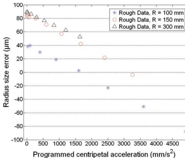
Fig. 8. Radius size error as a function of programmed centripetal acceleration for a horizontal circular path of various radii centred at approximately  $\{-290 \text{ mm}, 987 \text{ mm}, 615 \text{ mm}\}$ .
