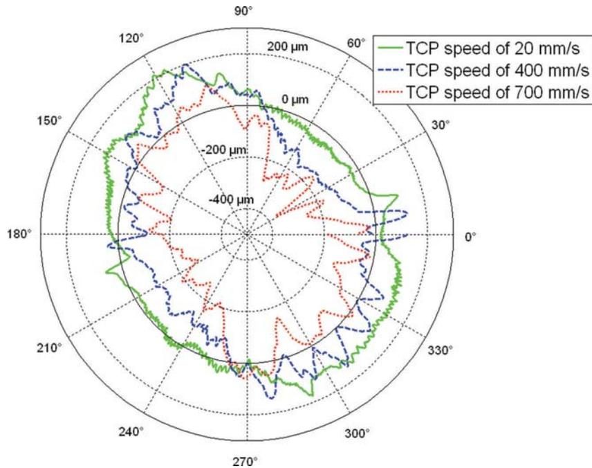
Fig. 7. Steady state contouring form errors in the CW direction for a horizontal circular path of radius of 100 mm and at TCP speeds of 20 mm/s, 400 mm/s and 700 mm/s, centered at approximately  $\{-290 \text{ mm}, 987 \text{ mm}, 615 \text{ mm}\}$ .
