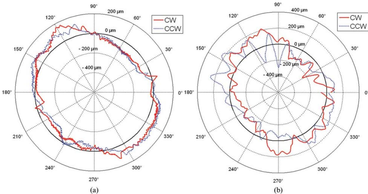
Fig. 2. Steady state contouring form errors in the CW and CWW directions for a horizontal circular path of radius 100 mm centred at approximately  $\{-290 \text{ mm}, 987 \text{ mm}, 615 \text{ mm}\}$ . (a) TCP speed of 30 mm/s. (b) TCP speed of 700 mm/s.
