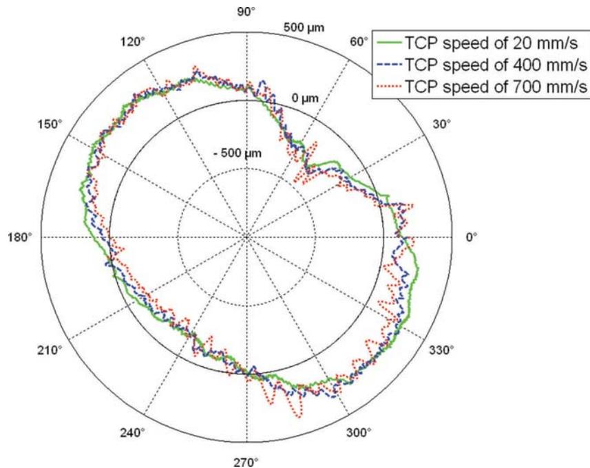
Fig. 5. Steady state contouring form errors in the CW direction for a horizontal circular path of radius of 300 mm and TCP speeds of 20 mm/s, 400 mm/s and 700 mm/s, centred at approximately  $\{-290 \text{ mm}, 987 \text{ mm}, 615 \text{ mm}\}$ .
