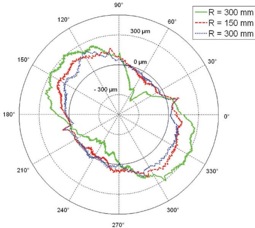
Fig. 6. Steady state contouring form errors in the CW direction for a horizontal circular path of radii 100 mm, 200 mm and 300 mm and at a TCP speed of 20 mm/s, centred at approximately  $\{-290 \text{ mm}, 987 \text{ mm}, 615 \text{ mm}\}$ .
