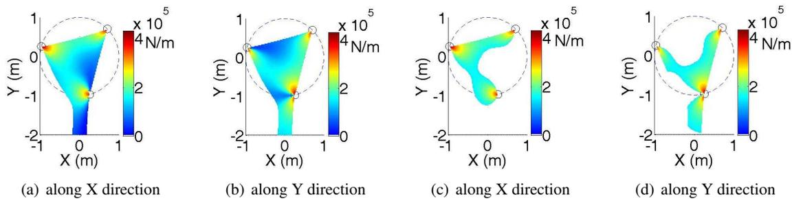
Fig. 2. Stiffness maps for a minimum stiffness  $K_{min}$  of: (a), (b) 0 kN/m; (c), (d) 150 kN/m.
