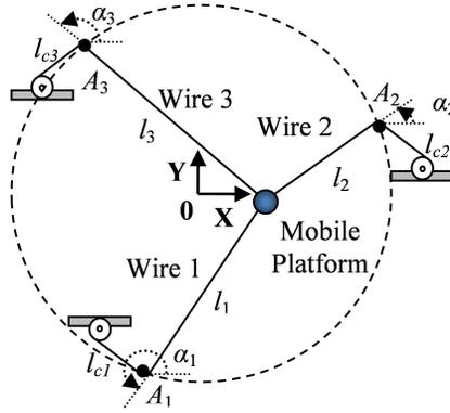
Fig. 1. Coordinate system and variables of 2 DOF planar three-wire-actuated parallel manipulators.
