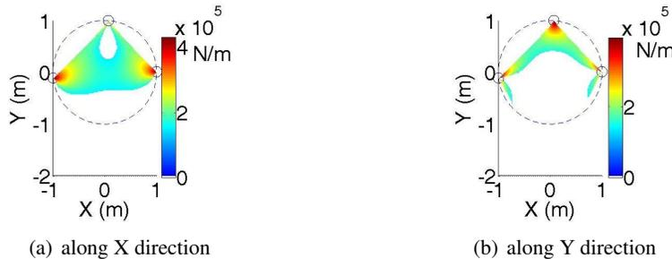
Fig. 5. Stiffness maps with optimum layout for  $K_{min} = 150 \text{ kN/m}$  in both  $X$  and  $Y$  directions.
