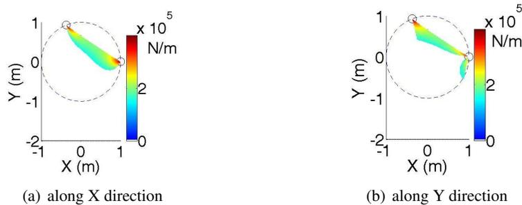
Fig. 7. Stiffness maps with optimum layout after failure of a wire for  $K_{min} = 150$  KN/m in both X and Y directions.
