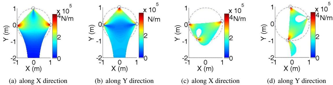
Fig. 4. Stiffness maps with optimum layout for  $K_{min}$  of: (a), (b)  $0 \text{ kN/m}$ ; (c), (d)  $150 \text{ kN/m}$ .
