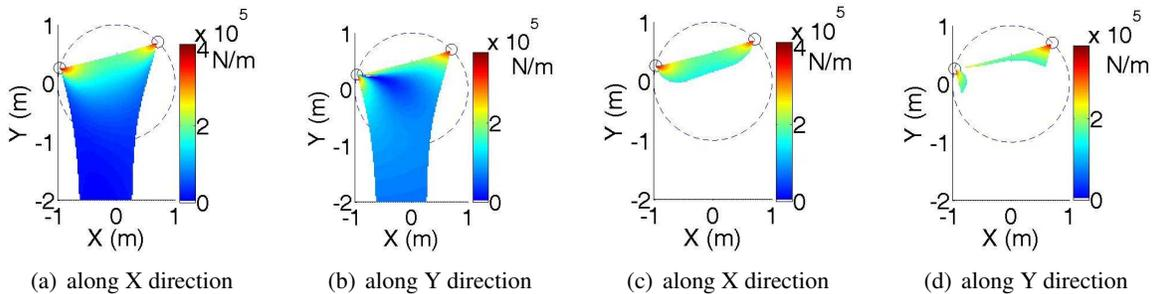
Fig. 3. Stiffness maps after failure of wire 1 for  $K_{min}$  of: (a), (b) 0 kN/m; (c), (d) 150 kN/m.
