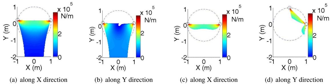
Fig. 6. Stiffness maps with optimum layout after failure of a wire for  $K_{min}$  of: (a), (b) 0 KN/m; (c), (d) 150 KN/m.
