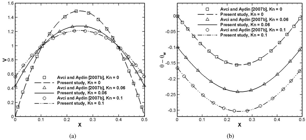
Fig. 2. Comparison of the fully developed (a) velocity and (b) temperature profiles with those of Avci and Aydin [6] at  $r_q = 1$ ;  $Gr/Re = 50$ ;  $Kn = 0, 0.06$  and  $0.1$ .
