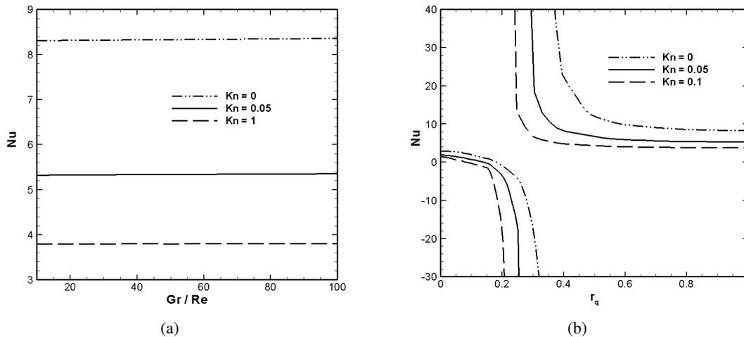
Fig. 9. The variations of the average Nusselt number with (a)  $Gr/Re$  for  $r_q = 1$ ; and (b)  $r_q$  for  $Gr/Re = 100$ , and different values of  $Kn$ .
