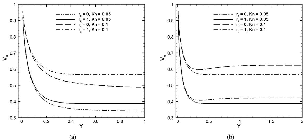
Fig. 6. Axial variations of slip velocities along (a) the cold wall; and (b) the hot wall for  $Gr/Re = 100$  and different values of  $r_q$  and  $Kn$ .
