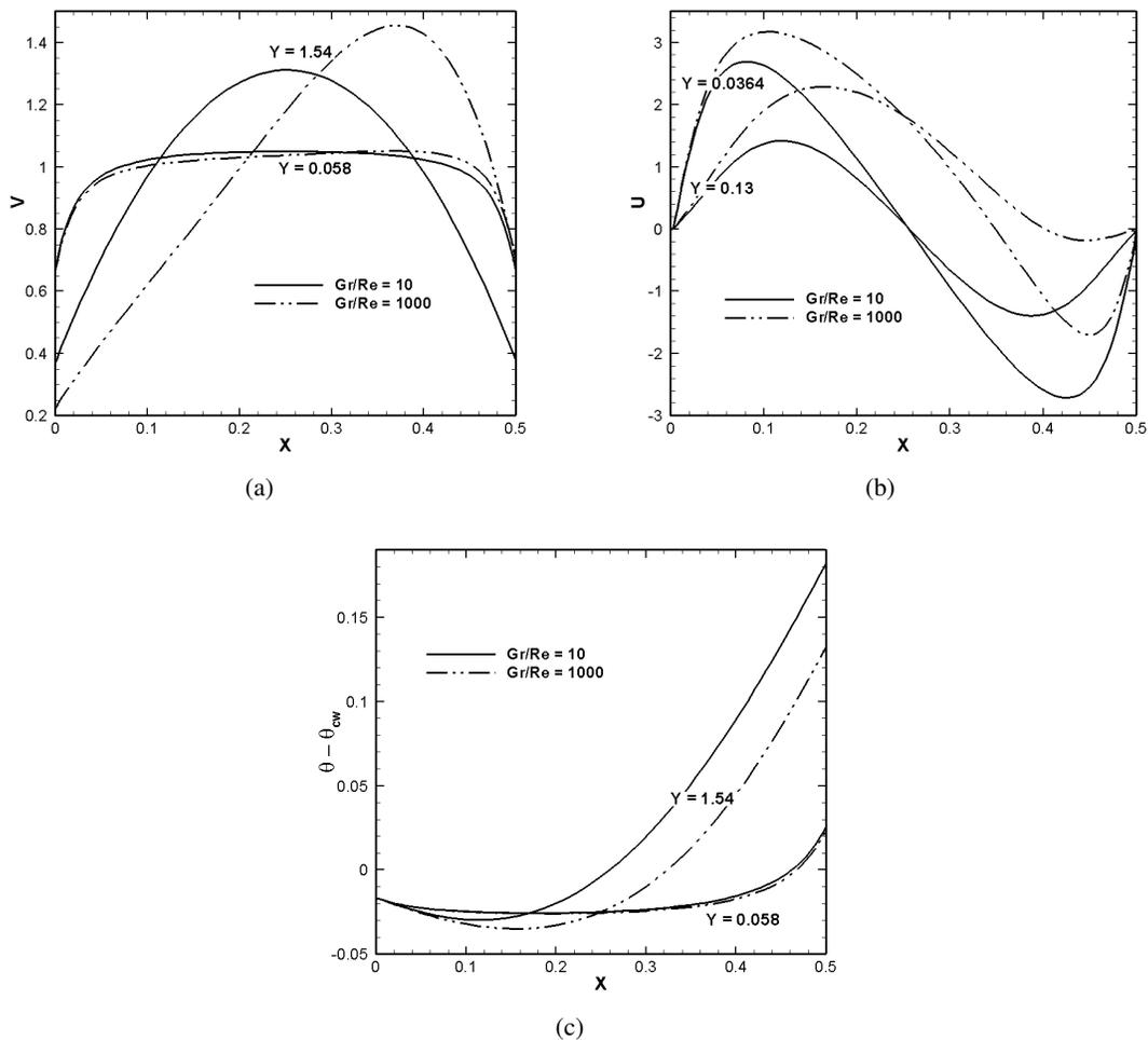
Fig. 8. Effects of mixed convection parameter on the (a) axial velocity; (b) cross flow velocity; and (c) temperature profiles for  $Kn = 0.05$  and  $r_q = 0.2$ .
