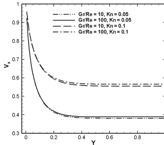
Fig. 5. Axial variations of slip velocities for  $r_q = 1$  and different values of  $Gr/Re$  and  $Kn$ .
