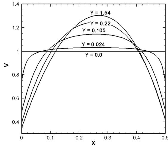
Fig. 3. Streamwise velocity profiles at different axial locations for  $Gr/Re = 100$ ,  $Kn = 0.05$  and 1.
