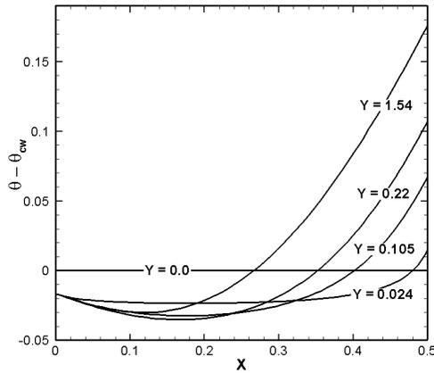
Fig. 7. Cross sectional temperature profiles at different axial locations for  $Gr/Re = 100$ ,  $Kn = 0.05$  and  $r_q = 0.2$ .
