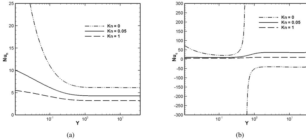
Fig. 10. Variations of local Nusselt number along (a) the hot wall; and (b) the cold wall for  $r_q = 0.3$ ,  $Gr/Re = 100$  and different values of  $Kn$ .
