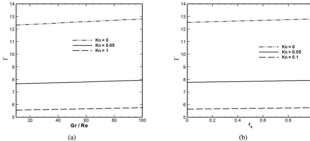
Fig. 11. The variations of the average friction coefficient with (a)  $Gr/Re$  for  $r_q = 1$ ; and (b)  $r_q$  for  $Gr/Re = 100$ , and different values of  $Kn$ .
