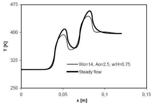
Fig. 6. The instantaneous temperatures along the wall for pulsating flow ( $Wo = 14$ ,  $A_0 = 2.5$ ,  $w/H = 0.75$ ) and steady flow conditions.
