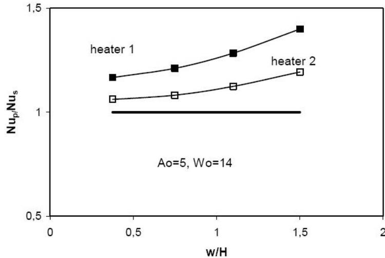
Fig. 12. The effect of distance between two heaters on the average Nusselt Numbers ( $A_0 = 5$ ,  $Wo = 14$ ).
