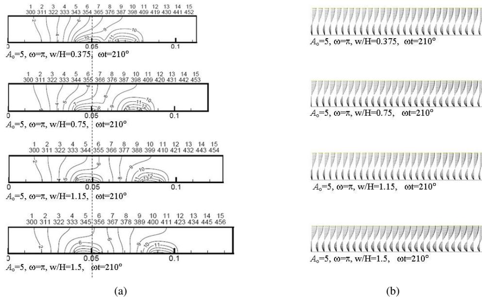
Fig. 11. (a) Temperature contours for different  $w/H$  at fixed frequency and specific phase angle ( $Wo \approx 14$ ), (b) Velocity vectors for situations in Fig. 11(a) ( $Wo \approx 14$ ).
