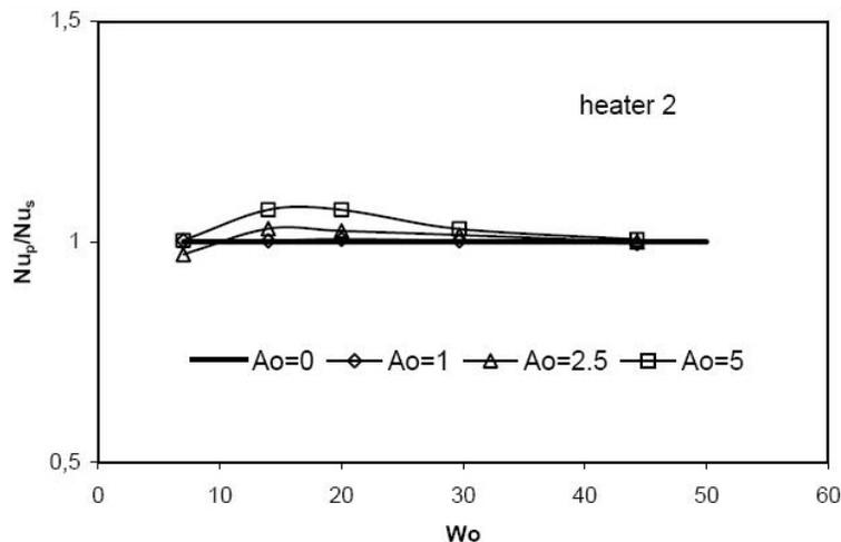
Fig. 10. Average Nusselt numbers versus dimensionless parameters for heater 2 ( $w/H = 0.75$ ).
