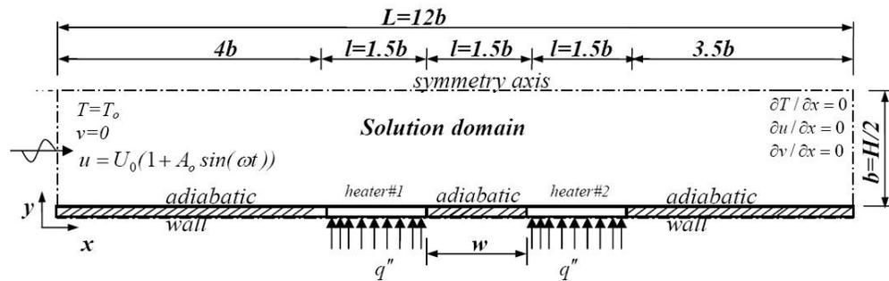
Fig. 1. Schematic view of flow domain and dimensions.
