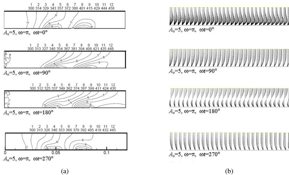
Fig. 5. (a) Temperature contours for various phase angles over a cycle ( $A_0 = 5$ ,  $Wo \approx 14$ ,  $w/H = 0.75$ ), (b) Velocity vectors for situations in Fig. 5(a), ( $A_0 = 5$ ,  $Wo \approx 14$ ,  $w/H = 0.75$ )
