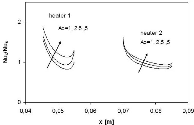
Fig. 8. Local Nusselt number along the discrete heaters ( $Wo = 20$ ,  $w/H = 0.75$ ).
