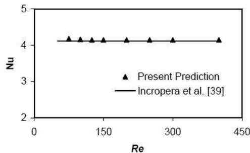
Fig. 3. Verification of Nu number with open literature [39].
