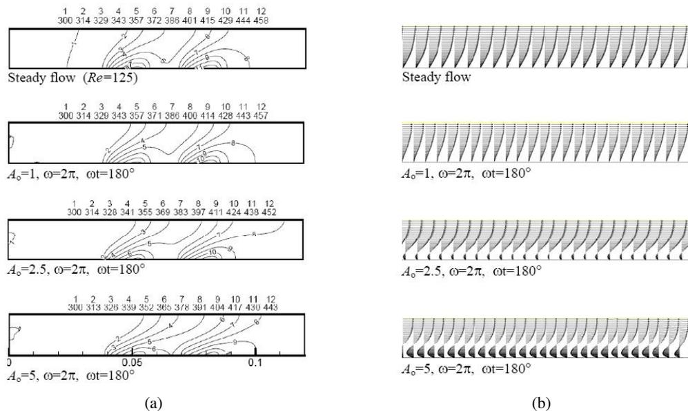
Fig. 4. (a) Temperature contours for different amplitude at fixed frequency and specific phase angle ( $Wo \approx 20$ ,  $w/H = 0.75$ ), (b) Velocity vectors for situations in Fig. 4(a), ( $Wo \approx 20$ ,  $w/H = 0.75$ ).
