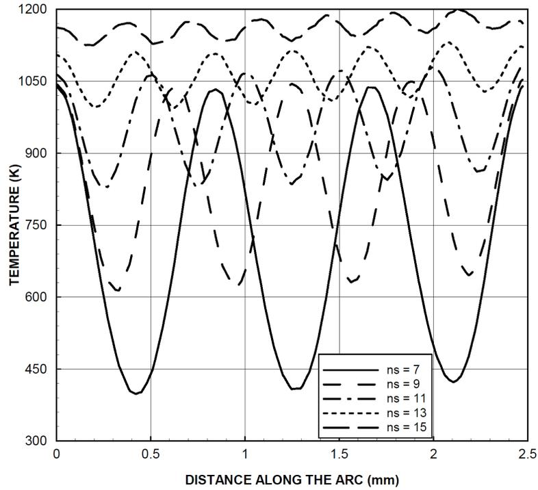
Fig. 3. Temperature distribution along the arc due to various number of spots. *ns* represents the number of spots.
