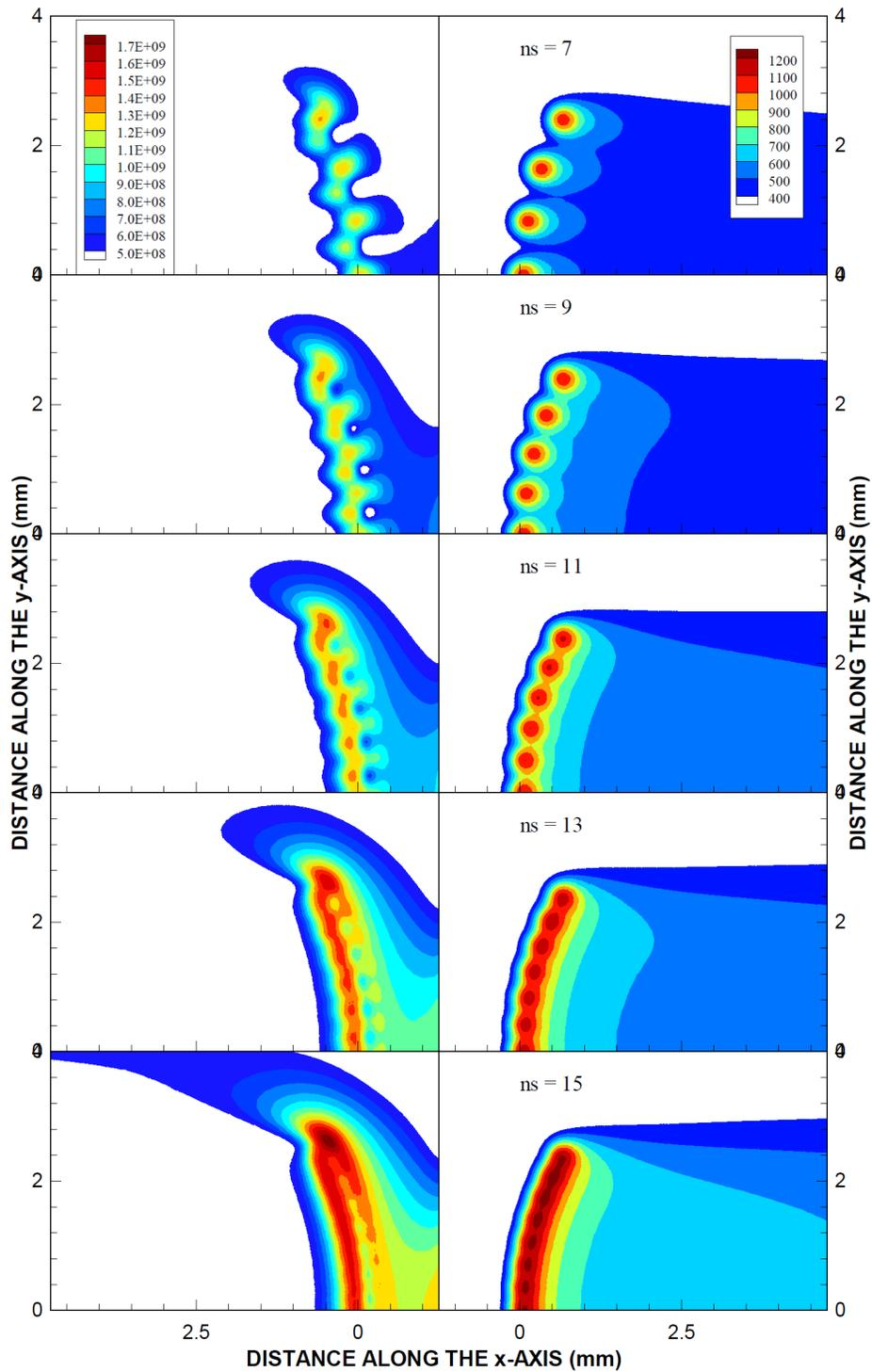
Fig. 2. Temperature and stress contours for various number of laser spots.  $ns$  represents the number of laser spots.
