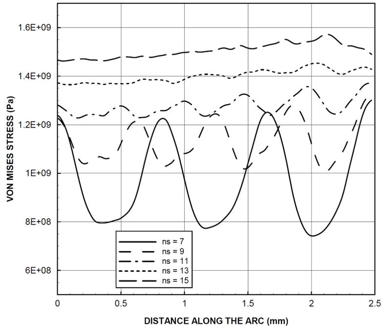
Fig. 4. von Mises distribution along the arc due to various number of spots. *ns* represents the number of spots.
