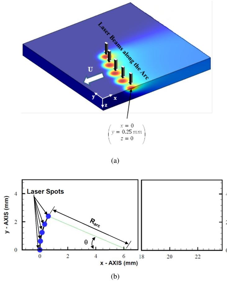
Fig. 1. A schematic view of laser spots along the arc: (a) the coordinate system, (b) top view of the workpiece and its size along with the laser spots.
