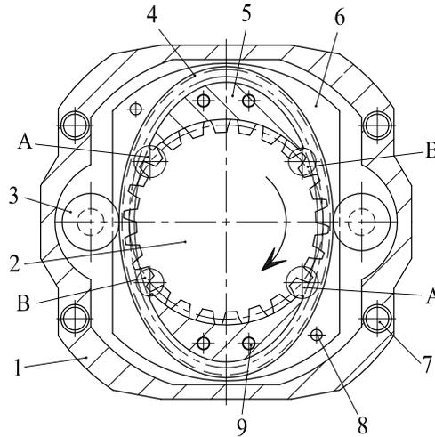
Fig. 1. Main parts of gear pump with flexible ring gear.
