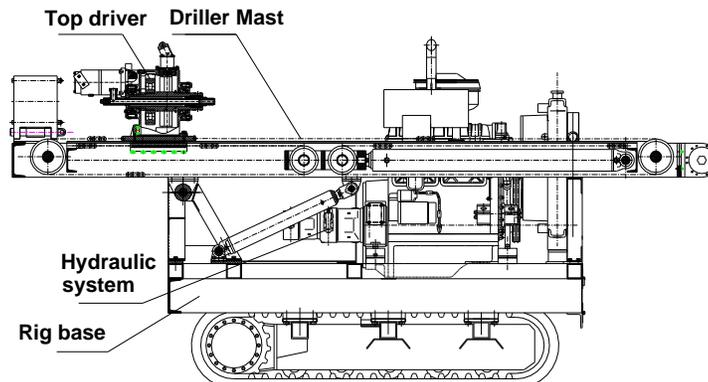
Fig. 2 Structure of sonic drill
