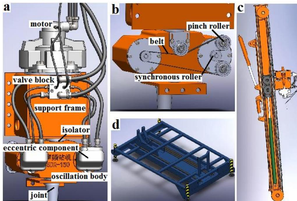
Fig. 3 Virtual prototype of a sonic driller
