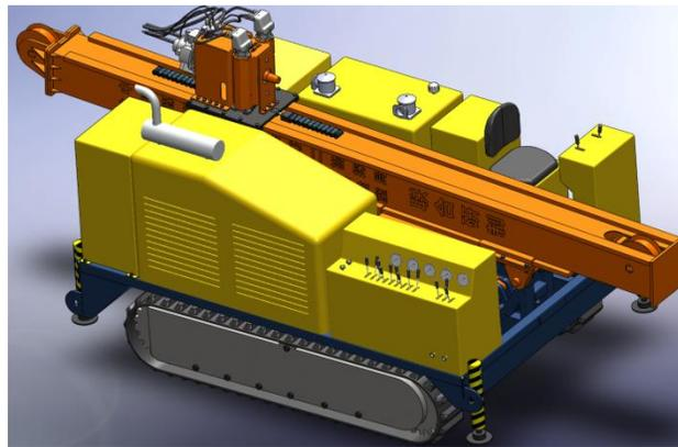
Fig. 4 Virtual prototype of sonic driller
