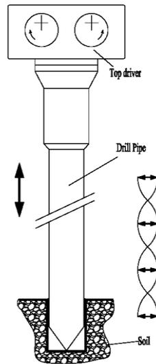
Fig. 1 Principles of sonic drilling processing
