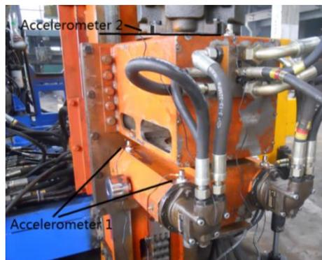
Fig. 8 Photo of vibration test
