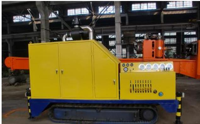
Fig. 7 photo of sonic driller prototype
