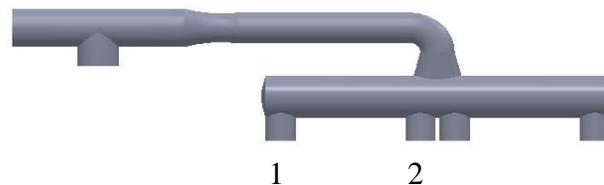
Fig. 2. The intake system consists of air duct, EGR and intake manifold.
