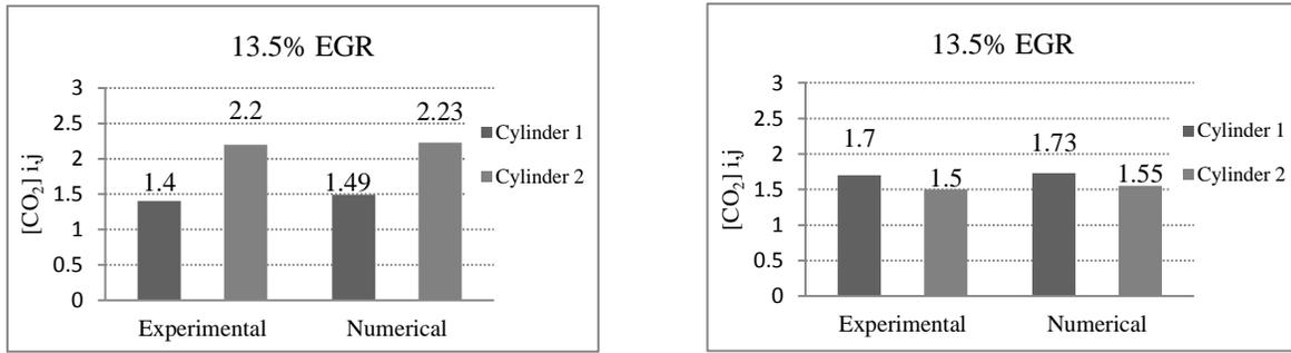
Fig. 3. CO<sub>2</sub> concentration at each inlet ports of cylinder 1 and 2 in cases of hot and cooled EGR for various EGR rates (continued).
