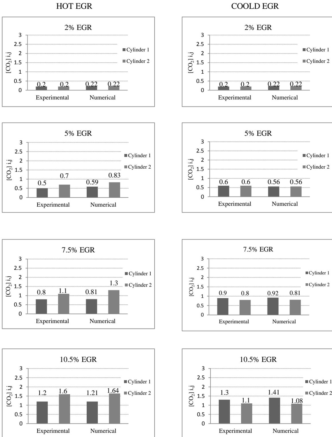
Fig. 3. CO<sub>2</sub> concentration at each inlet ports of cylinder 1 and 2 in cases of hot and cooled EGR for various EGR rates (continues).
