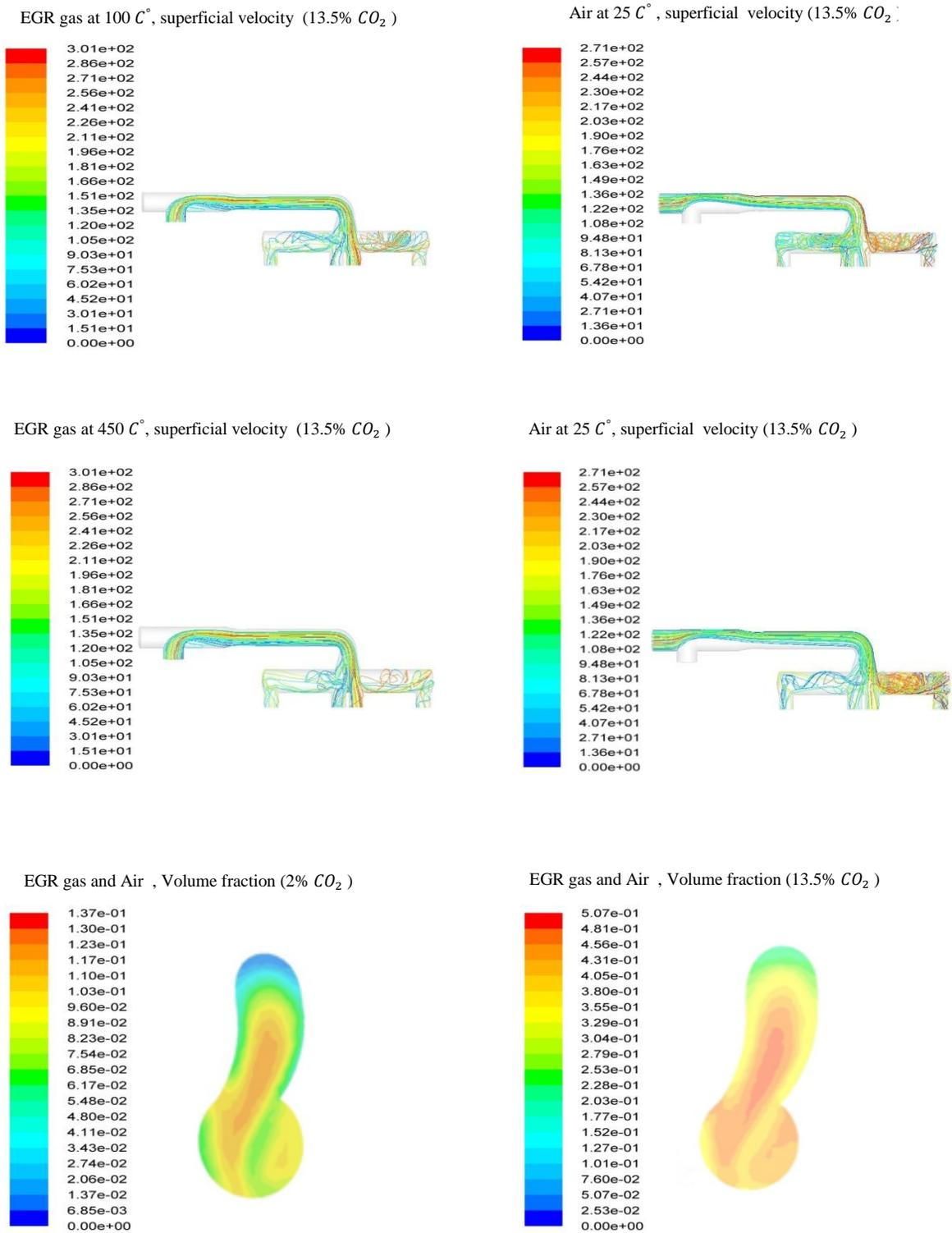
Fig. 4. Stream line and volume fraction of air and EGR gas at various percentages of CO<sub>2</sub> (continued).
