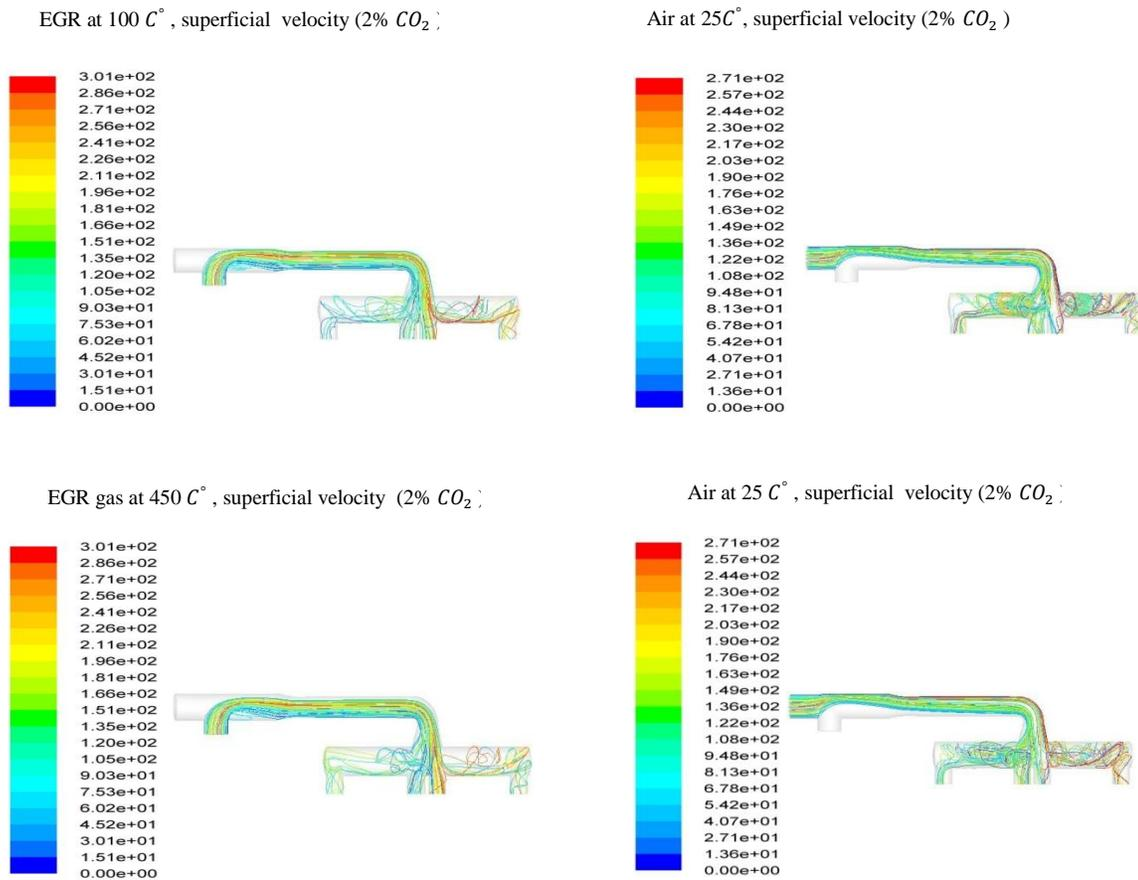
Fig. 4. Stream line and volume fraction of air and EGR gas at various percentages of CO<sub>2</sub> (continues).
