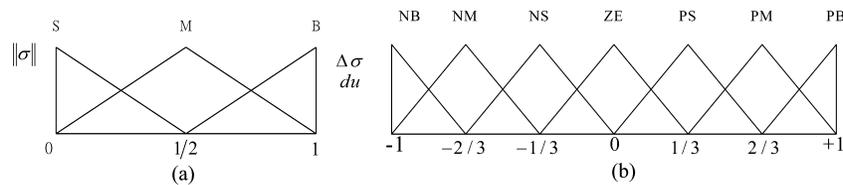
Fig. 3. Membership function (a)  $\|\sigma\|$ ; (b)  $\Delta\sigma$  and  $du$ .
