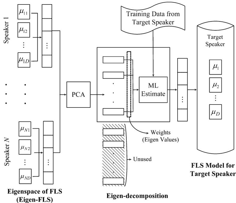
Fig. 1. Eigenspace-based FLS (Eigen-FLS) frameworks for speech pattern recognition.
