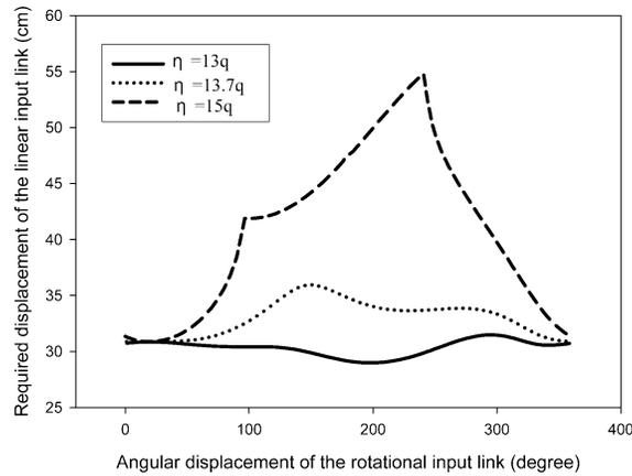
Fig. 6. The required displacements of linear input link corresponding to the current angular displacements of rotational input link for Example 2.
