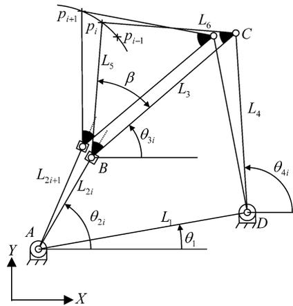
Fig. 2. The coordinate system of the new programmable exact path generator.
