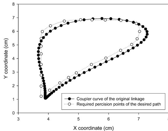
Fig. 3. Precision points of the required path and coupler curve of the original linkage.
