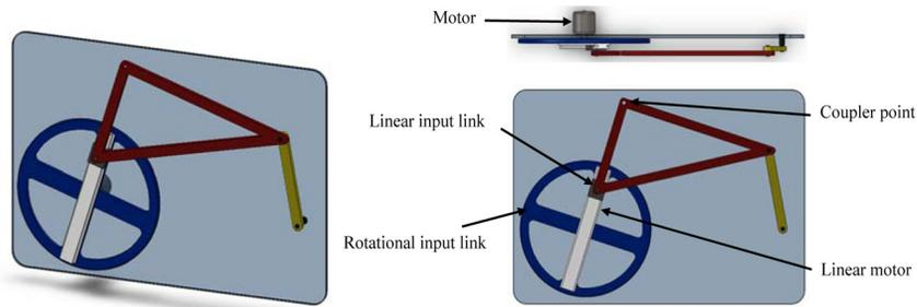
Fig. 1. The new programmable exact path generator.
