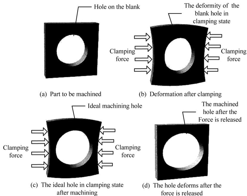
Fig. 2. Machining error caused by the clamping force.
