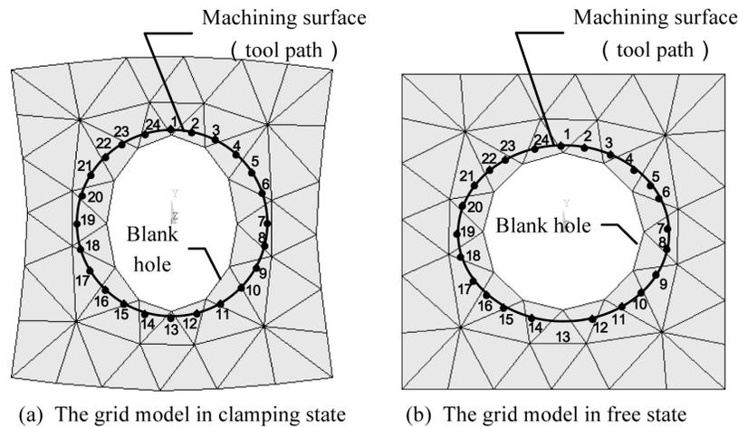
Fig. 3. The variation of track points in the grid model before and after releasing the clamping force.
