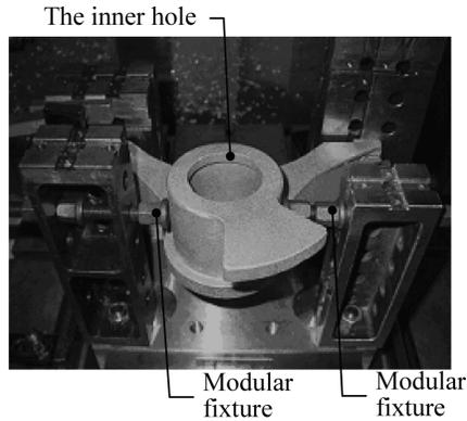
Fig. 1. The case of accuracy affected by the clamping force.
