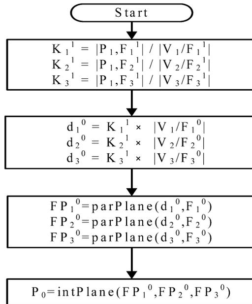
Fig. 7. The tetrahedral mapping algorithm flow of the point P1.
