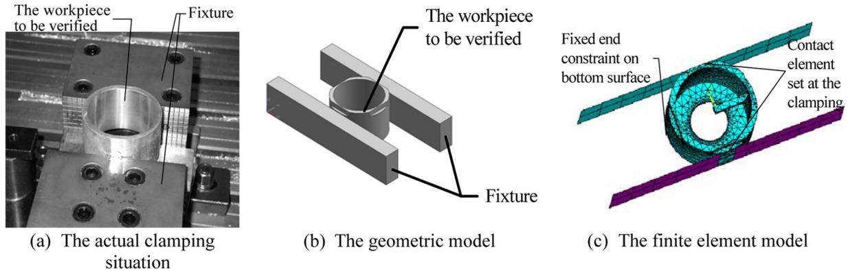
Fig. 8. The workpiece for verification.
