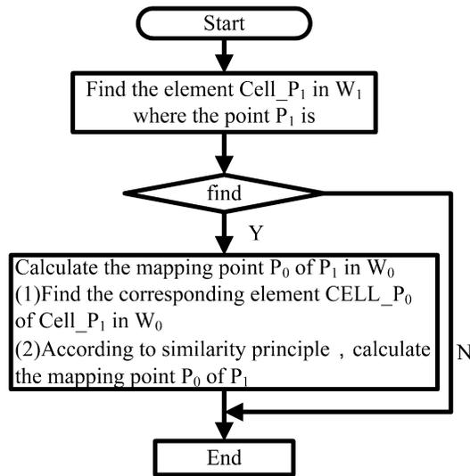
Fig. 5. The mapping algorithm to arbitrary point P1 based on grid.
