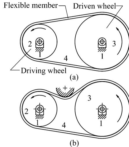
Fig. 2. A flexible connecting mechanism.
