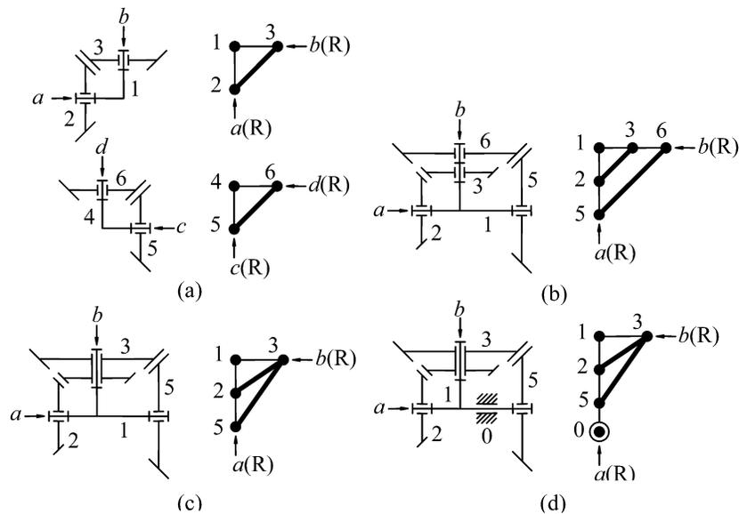
Fig. 4. Composition and decomposition of mechanisms.
