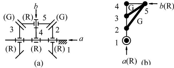
Fig. 1. A typical differential mechanism.
