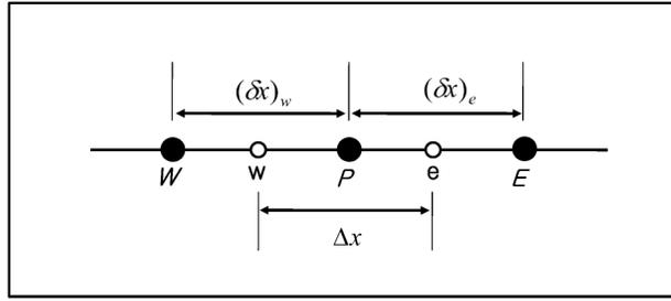
Fig. 2. Grid points for finite volume method in 1-D coordinates.
