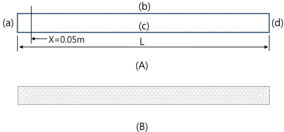
Fig. 4. Geometry of numerical simulation. The boundary conditions are (a)  $-n \cdot (-k\nabla T) = q_0 = 150 \text{ [W/m}^2\text{]}$ , (b)  $-n \cdot (-k\nabla T) = 0$ , (c)  $-n \cdot (-k\nabla T) = 0$  and (d)  $n \cdot (-k\nabla T) = 0$  for (A).  $L = 3 \text{ m}$  is longer than a measurement point  $X$  and  $X$  is a measurement point with time. The number of elements is 2049 for (B).
