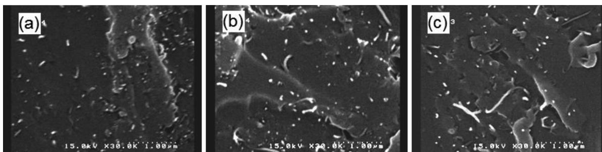
Fig. 3. SEM images of the fracture surfaces for the specimens with 0.5 wt.% CNTs statically tested at (a) RT/MH, (b) RT/HH, and (c) HT/HH environments ( $\times 30,000$ ).
