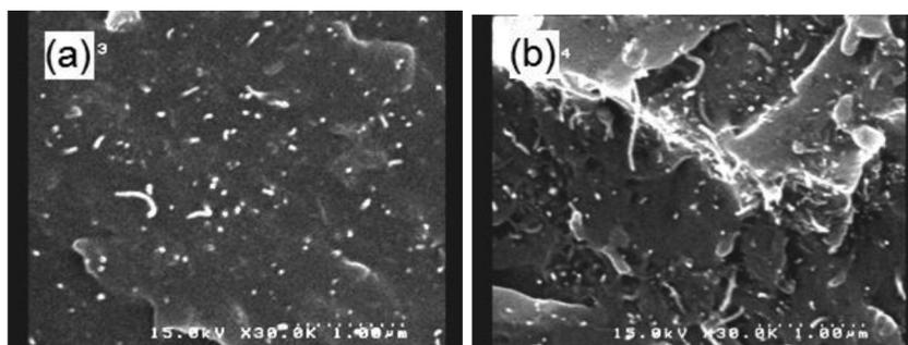
Fig. 4. SEM images of the fracture surfaces for the specimens with (a) 0.5 and (b) 1.0 wt.% CNTs statically tested at RT/MH environments ( $\times 30,000$ ).
