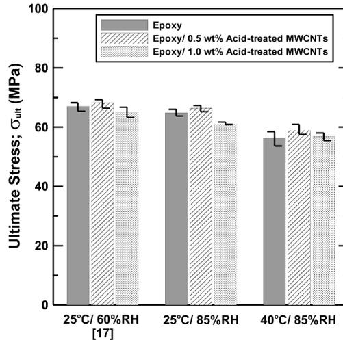
Fig. 2. Effects of hydrothermal conditions and CNT contents on the ultimate strengths of the CNT/epoxy composites.
