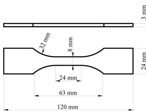
Fig. 1. Shape and dimensions of the studied CNT/epoxy specimen.
