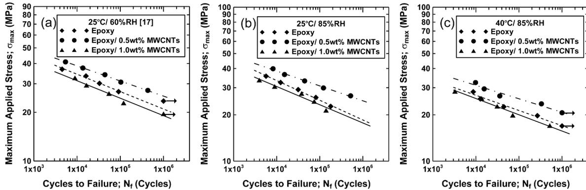
Fig. 6. Experimental results of the fatigue tests and corresponding stress-life curves for the CNT/epoxy composites with various CNT contents under (a) RT/MH, (b) RT/HH, and (c) HT/HH hydrothermal conditions.
