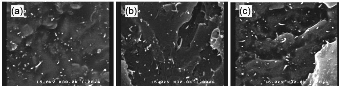
Fig. 7. SEM images of the fracture surfaces for the specimens with 0.5 wt.% CNTs fatigue-tested at (a) RT/MH, (b) RT/HH, and (c) HT/HH environments ( $\times 30,000$ ).
