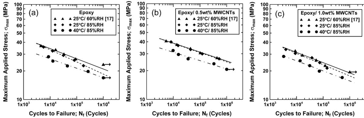
Fig. 5. Experimental results of the fatigue tests and corresponding stress-life curves for the CNT/epoxy composites with (a) 0, (b) 0.5, and (c) 1.0 wt.% CNT contents under various hydrothermal conditions.
