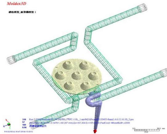
Fig. 1. Mesh model of injection molding.
