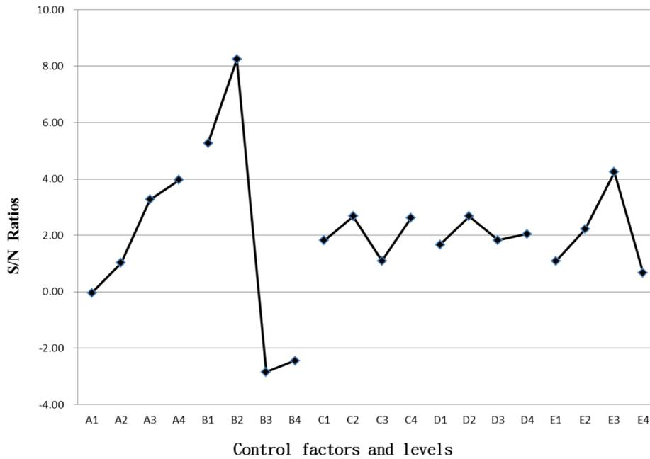
Fig. 6. Response diagram for shrinkage.
