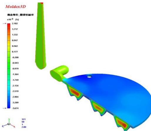
Fig. 2. Volumetric shrinkage.
