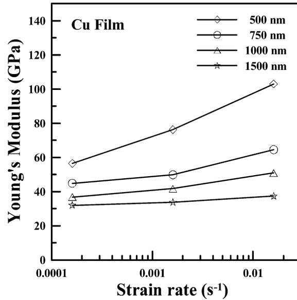
Fig. 5. The relationship between the Young's modulus and the strain rate with various thicknesses of Cu films.
