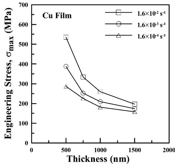
Fig. 6. The relationship between the maximum stress and the thicknesses of Cu films  $t$  with various strain rates.
