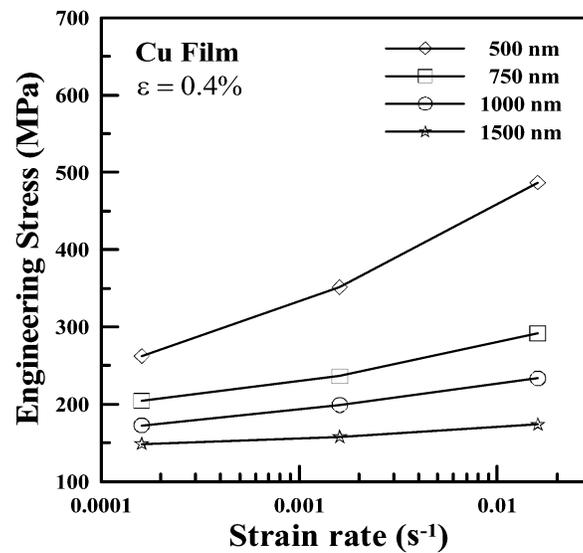
Fig. 8. Variations of shear stress with strain rate at a strain of 0.004 under different thicknesses of Cu film conditions.
