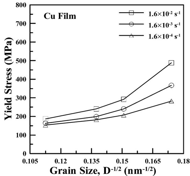
Fig. 11. Variations of the yield stress as a function of grain size  $D^{-1/2}$  under different strain rate conditions.
