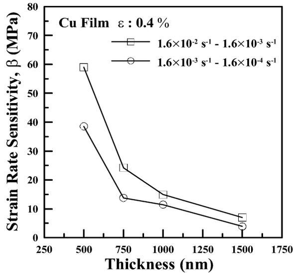
Fig. 9. Variations of the strain rate sensitivity parameter  $\beta$  with the strain as a function of the thickness of Cu film and strain rate.
