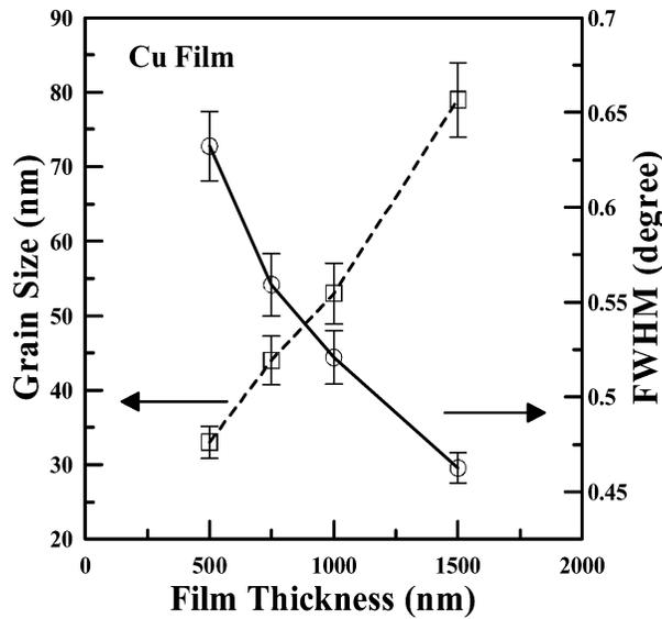
Fig. 10. The relationship between gain size and the thickness of Cu film.
