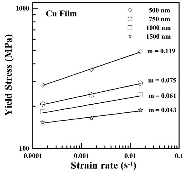
Fig. 7. The logarithmic plot of the relationship between the yield stress and the strain rate with various thicknesses of Cu films.
