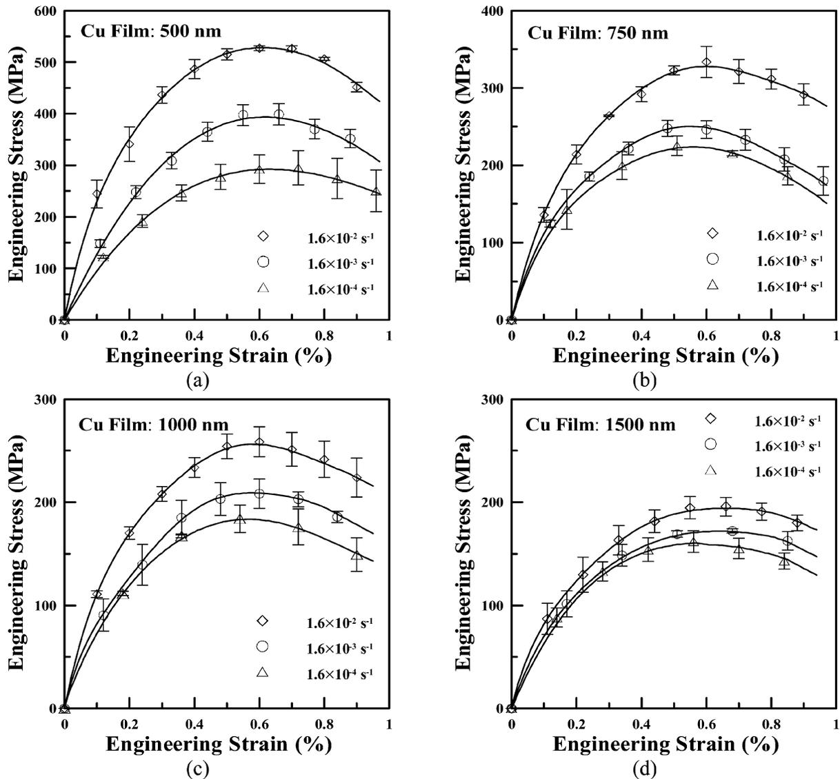
Fig. 3. The relationship of stress-strain of Cu thin film with (a) 500 nm; (b) 750 nm; (c) 1000 nm; (d) 1500 nm thickness under various strain rates.
