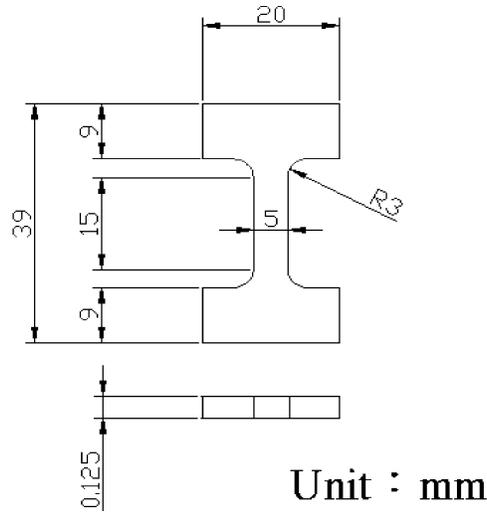
Fig. 1. Dimension of tensile test vehicle.
