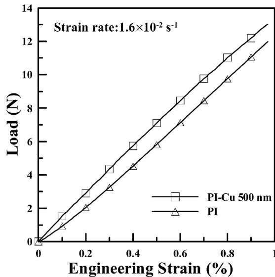
Fig. 2. The relationship of load and strain of deposited Cu and PI film under a strain rate condition.
